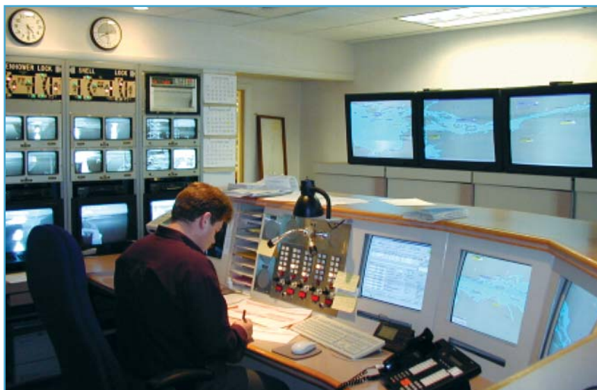
The Volpe Center recently implemented a vessel communications and tracking network for the Saint Lawrence Seaway. The network, based on the automatic identification system, promises improved safety, security, and efficiency throughout the Seaway. Above, the new system in use at the Eisenhower Lock vessel traffic control center in New York. (Photo courtesy of Mr. Kam Chin)
