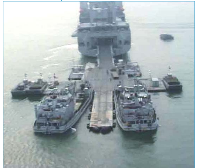
The Roll-on/Roll-off Discharge Facility is a floating platform that provides a roadway between a ship's ramp and a powered ferry. (Photo courtesy of Mr. Michael Buonopane)
