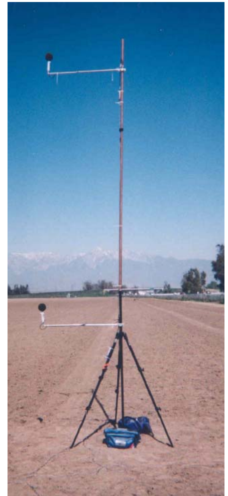
Microphones capture highway traffic noise for the FHWA’s Traffic Noise Model validation study.
