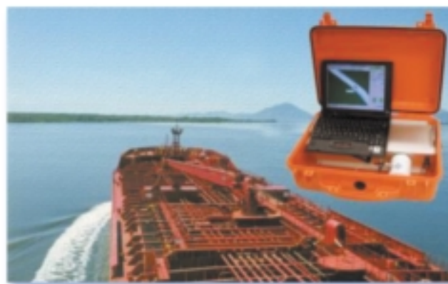
Each onboard navigation system consists of a laptop computer, radio-beacon antenna, and GPS receiver.
