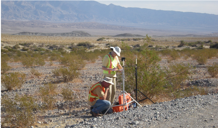
Volpe researchers set up acoustic equipment to measure wayside noise in Death Valley.
