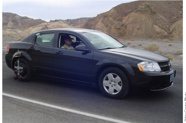
Vehicle outfitted to gathering TNM noise data in real-world conditions.
