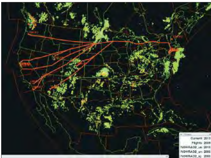
The Re-Route Impact Assessment tool displays a re-route around convective weather.
