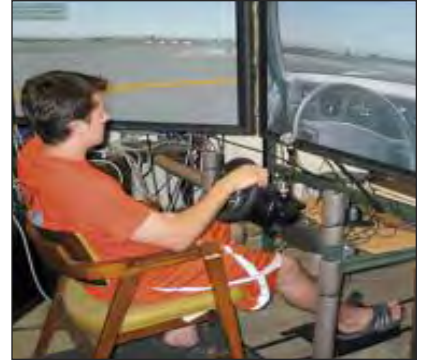
Summer Transportation Institutes student testing the Airport Surface Low-Cost Driving Simulator in the Volpe Center's Human Factors Laboratory.
