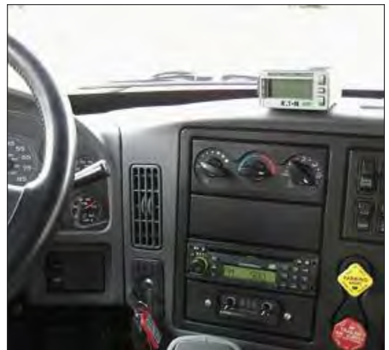
IVBSS driver-vehicle interface in a heavy truck platform.
