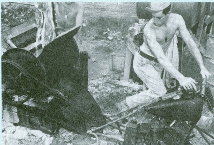
A 'Rube Goldberg' machine built from a steel drum and an old motorcycle
