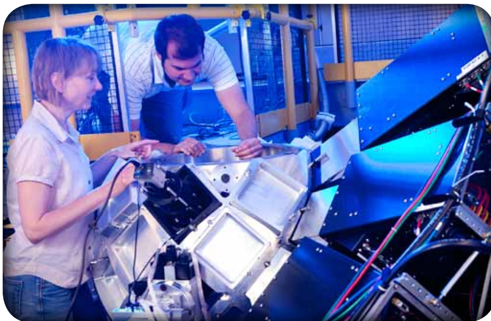
Christina Hoffmann, lead instrument scientist, and Matt Frost, scientific associate, work on TOPAZ, a new single-crystal diffractometer at SNS. TOPAZ will greatly expand the range of materials that can be studied in biology, chemistry, earth sciences, materials, and solid-state physics.
