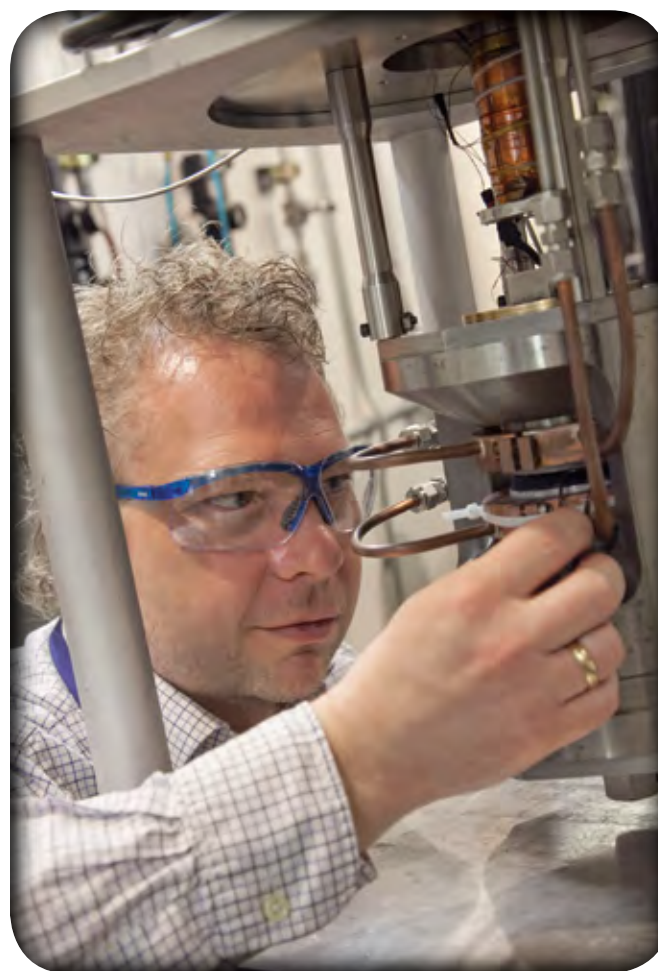
Chris Tulk aligns a sample in a Paris-Edinburgh press in preparation for a low-temperature, high-pressure experiment. Tulk and collaborators are engaged in new research on clathrate hydrates.
