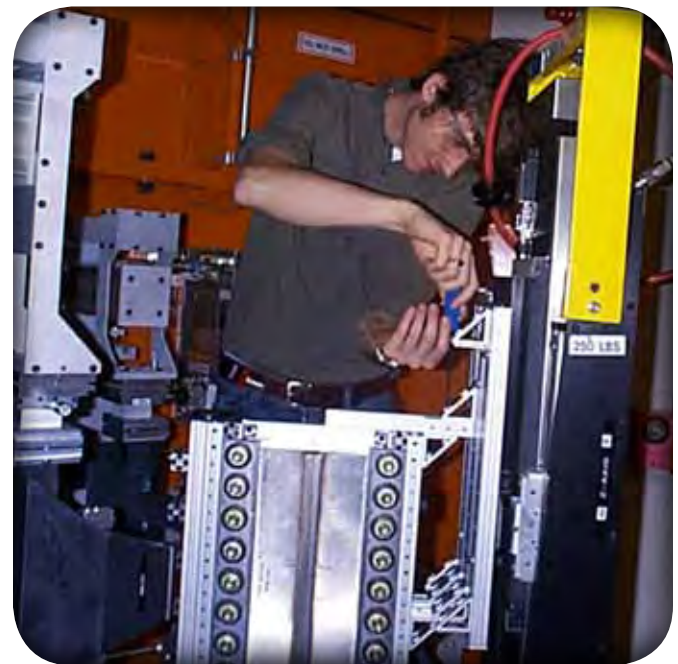
Matt Klug from Dominion Engineering, a subcontractor to EPRI, uses NSRF-2 to study stress distributions in joints welded to PWRs, helping to project crack growth and the probability of failure in the welds.
