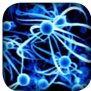
CNMS: Gallium ball-Si crystal-SiO x nanowire octopus.
