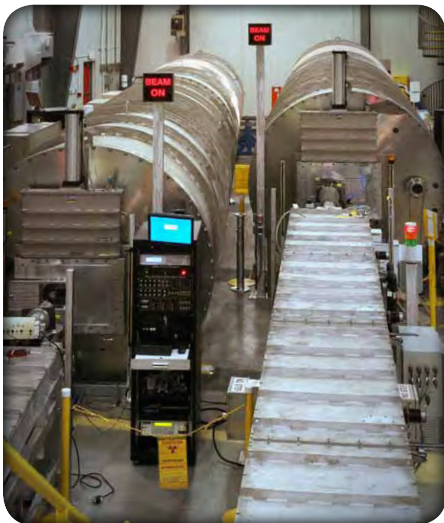
Detector tanks for the SANS instruments at HFIR. The Bio-SANS tank is on the right. On the left is the tank for the General-Purpose SANS instrument.
