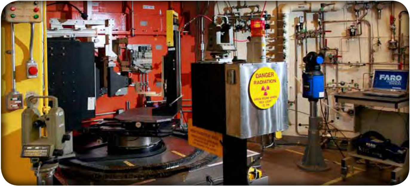
The Neutron Residual Stress Facility maps hidden stresses that affect the performance of materials.
