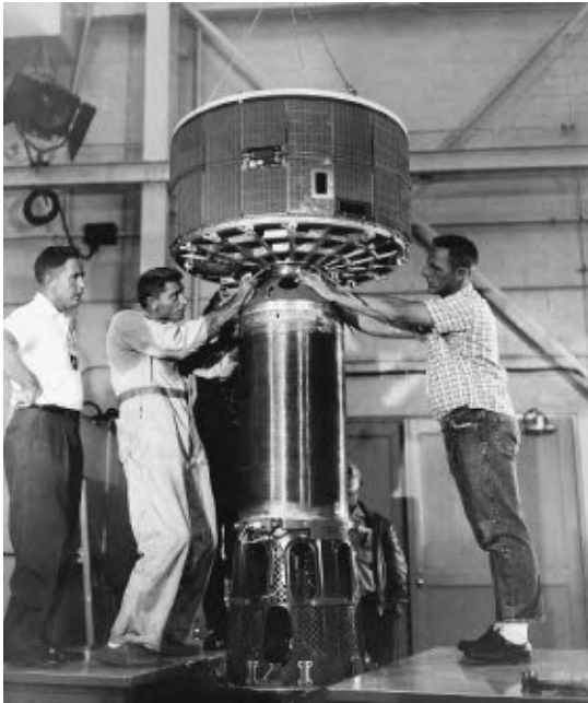
Workers putting the finishing touches on the nation’s first weather satellite, the Television Infrared Observation Satellite (TIROS), which launched from Cape Canaveral on 1 April 1960. The satellite weighed 270 pounds and carried two television cameras, a magnetic tape recorder, timer systems, transmitters, and a power supply. Early photographs provided new information on cloud systems, including spiral formations associated with large storms.
