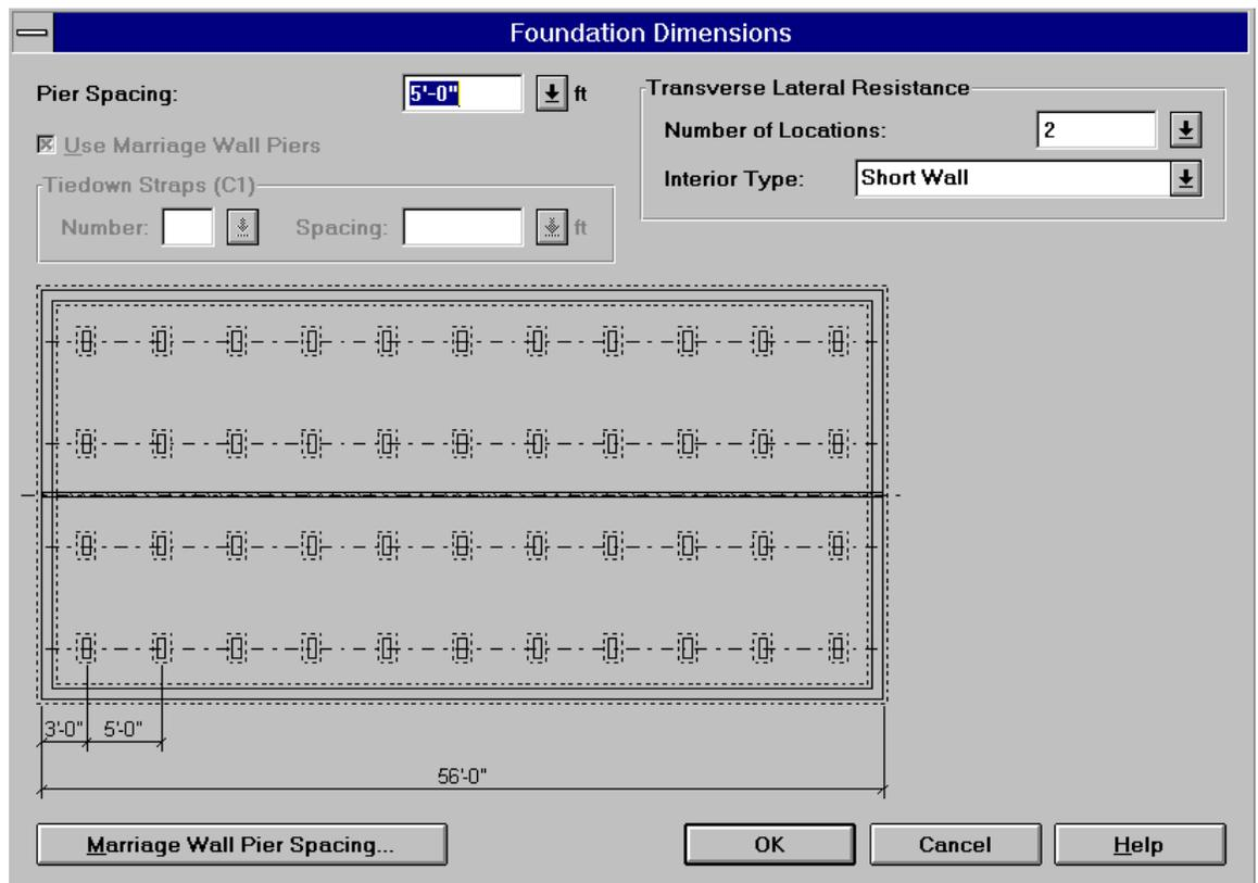
Note that at this point no marriage wall piers are shown. The User should select the “Marriage Wall Pier Spacing” button to bring up the **Marriage Wall Pier Spacing** dialog window as shown below:
