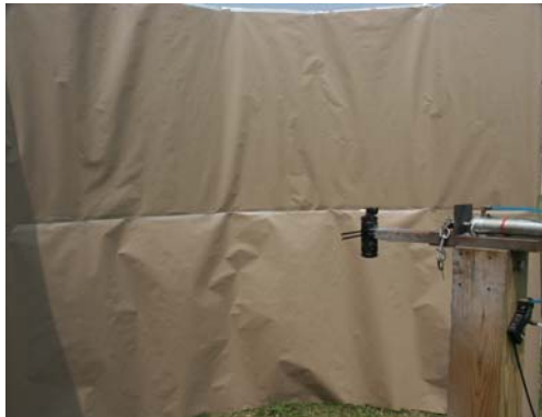
Figure 7. Set-Up of Fragmentation Arena – Fixturing and Witness Panels
