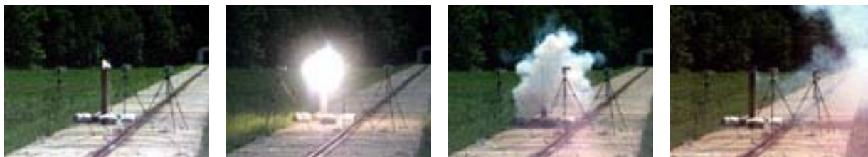
Figure 1. Digital SLR Camera Frame Sequence (Partial) of NFDD Fireball Growth and Decay
