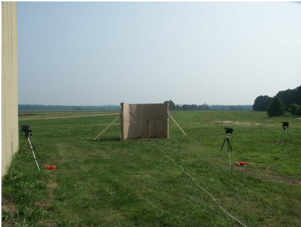
Figure 12. Example Fragmentation Arena – Pre-Test
