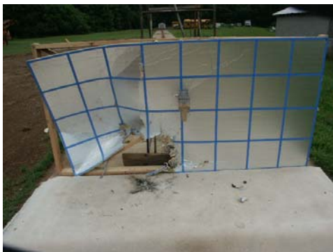
Figure 8. Witness Panel Damage Due To Confinement of NFDD between Test Object and Panel
