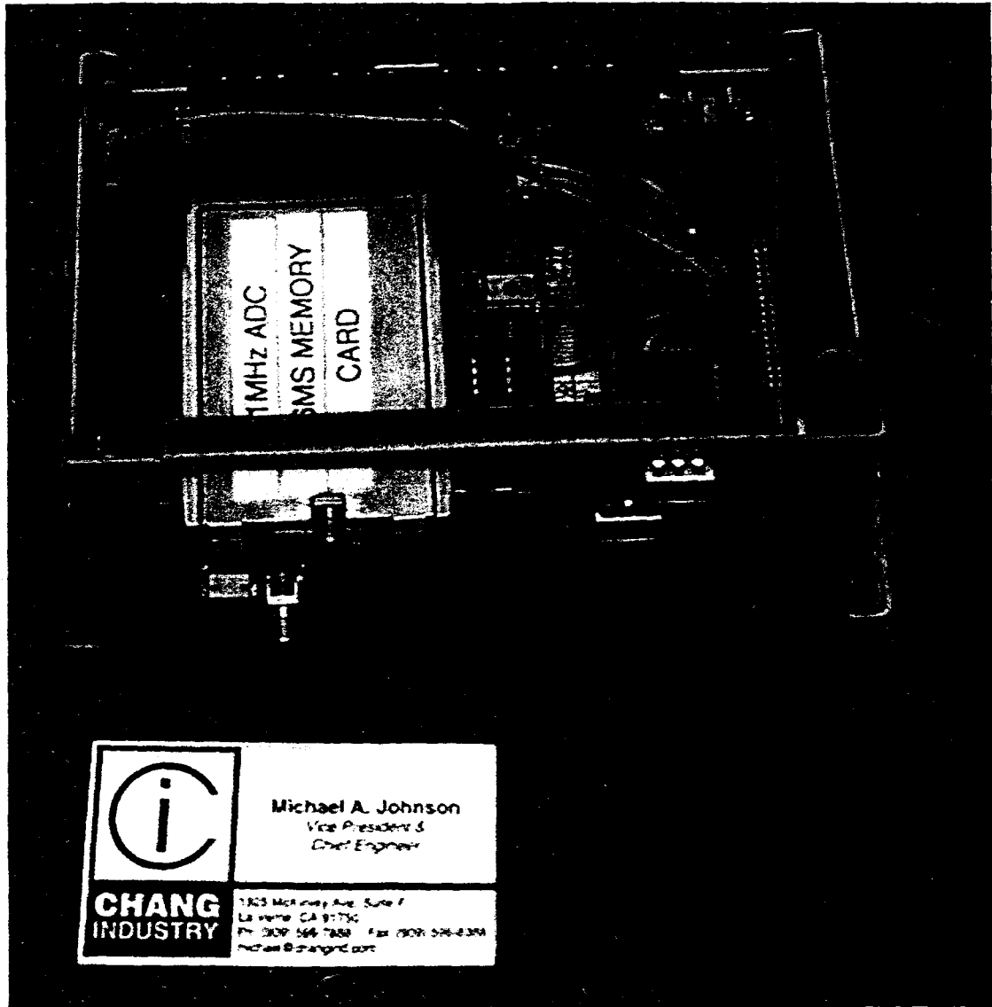
Figure 3.6 Data Acquisition System (Installed)
