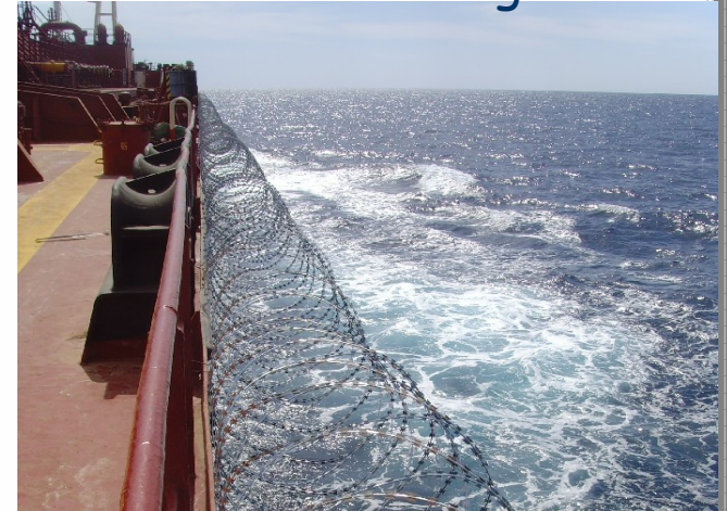
Barbed wire installed
