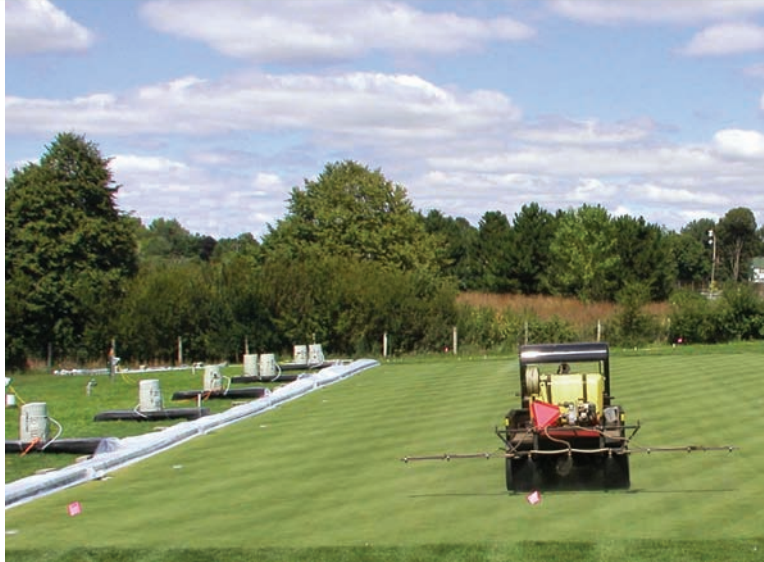
Pesticides being applied to experimental turf plots maintained at a golf course fairway. Following a simulated rain event, runoff was collected from the plots and analyzed for five different pesticides.
