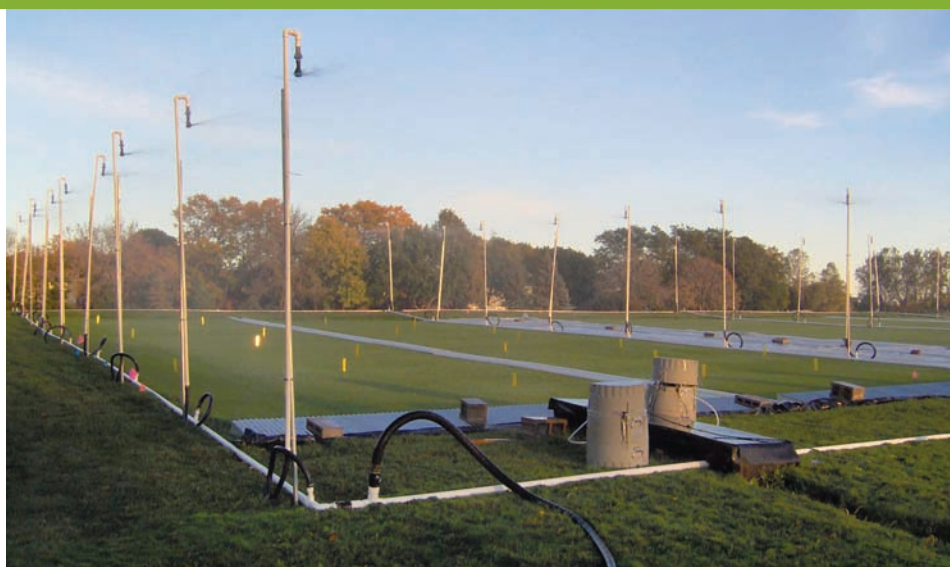
At the University of Minnesota Turf Research, Outreach, and Education Center in St. Paul, Minnesota, a rainfall simulator is used to generate runoff. Plots were equipped with rain gauges and automated runoff samplers to measure precipitation, runoff, and flow rates, and to collect periodic runoff samples.
