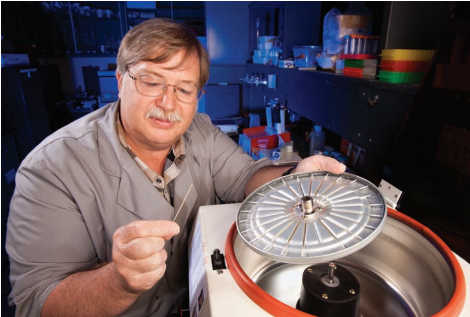
Technician Mike Judy loads immunoglobulin immunocrit tubes into a centrifuge. After centrifugation, the immunocrit measurement is easily made with a metric ruler.
