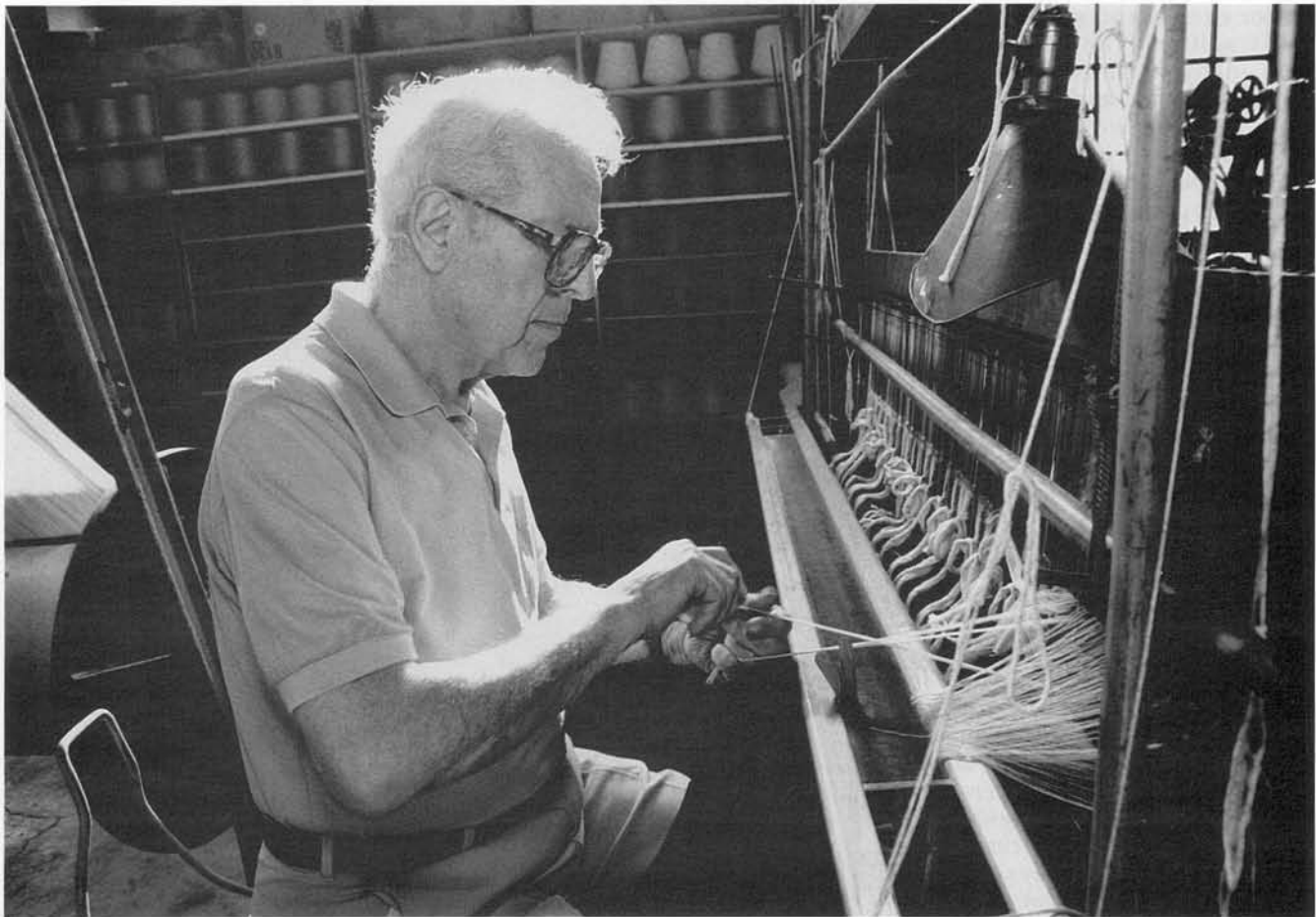
Sam Balister, the resident textile expert at the Paterson Museum, demonstrates how to pull warp ends through the reed of a weaving apparatus called an "entering frame." Balister worked in Paterson's textile industry for over forty years and became a master "twister"—the person responsible for joining (twisting together) the individual threads ("ends") of two warps on a loom. (WIP-MC-B031-10) Photo by Martha Cooper
