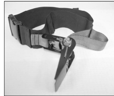
Fig 6. The LRT. The metal portion (similar to a cargo strap) contains a cam-and-ratchet device to tighten the outer strap. This device malfunctioned in some trials.
