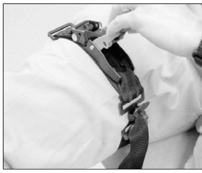
Fig 2. SATS. The cam system used in this tourniquet provided too little excursion to reliably and effectively occlude blood flow.
