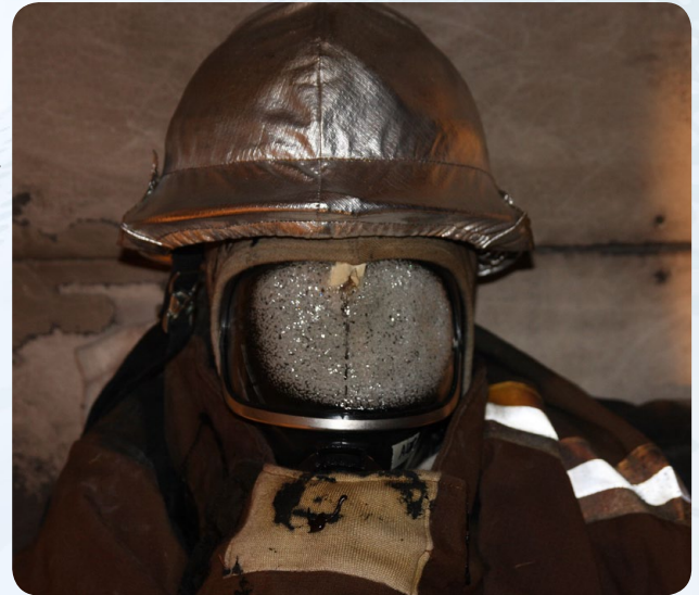
An SCBA face piece, shown with other components of fire fighter protective equipment mounted on a instrumented mannequin, after a full scale fire experiment in the Large Fire Research Facility
