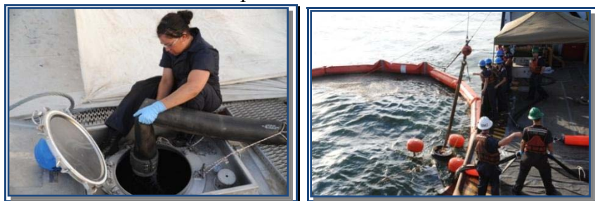
Source: USCG. Left – A USCG crewmember monitors a hose transporting an oil-and-water mix from the Spilled Oil Recovery System to a 4,200-gallon tank onboard the USCG Cutter Juniper on June 11, 2010.
