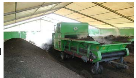
Composting TNT contaminated soil
