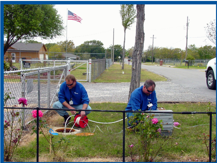
Contractor personnel collect water samples from a monitoring well located in the Tinker View Acres neighborhood
