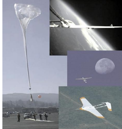
Figure 12. An Example Hybrid Balloon/UAV Platform. 165 Clockwise from upper right: glider flying at 100,000 ft shot from tail boom; two different gliders in flight; and launch of glider/payload (glider wings folded) under a standard balloon.
