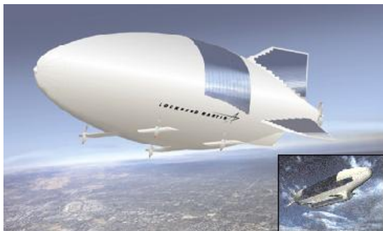
Figure 16. The Army's High Altitude Airship ACTD. Inset: conceptual production version. 182
