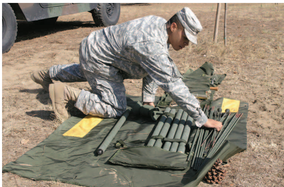
Sgt. Emmanuel Campos, 2nd Platoon, 13th MP Company, prepares to assemble a OE-254 antenna as part of the two weeks training at Camp Darby
