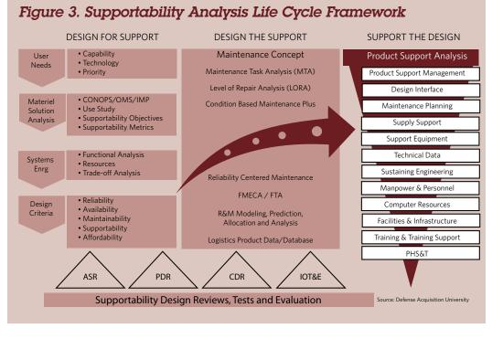
analysis; failure mode, effects and criticality (FMECA); fault tree analysis (FTA); and condition-based maintenance plus (CBM+), and reliability centered maintenance (RCM).
