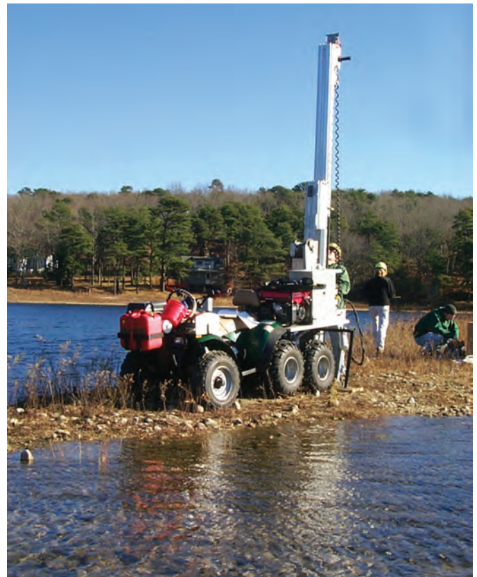
Figure 3. Photograph of drive-point drilling rig on the intermittent island in Snake Pond, Sandwich, Massachusetts, November 25, 2003.
