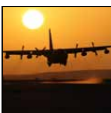
DJIBOUTI - An HC-130 P/N King carrying Air Force Reservists lands on an unimproved air strip after a mission to provide rescue support. The HC-130s provide an extended-range refueling capacity to helicopter rescue units operating in the area. (U.S. Air Force Photo/Master Sgt. Rob Grande)
