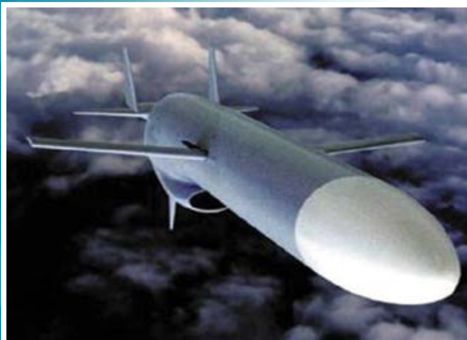
MALD, a low-cost, air-launched, programmable craft that accurately duplicates combat flight profiles and signatures of US and allied aircraft.
