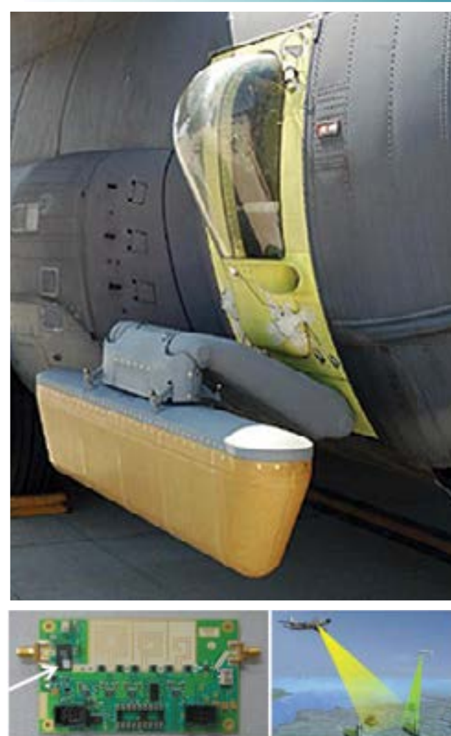
L3 Miniature Reconfigurable Beamformer with AFRL TTD module integrated with an antenna into an aircraft pod. (pictured top) L3 Miniature Reconfigurable Beamformer with AFRL TTD module. (pictured left) Simulation of an aircraft searching for signals of interest, showing reach of TTD module. (pictured right)
