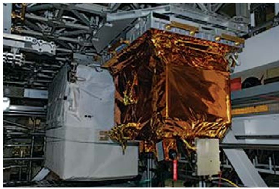
AFRL's VADER, 1 of 2 thermal management experiments to more efficiently control and manage heat transfer. VADER and MHTEX were included in this year's Endeavor shuttle flight.
