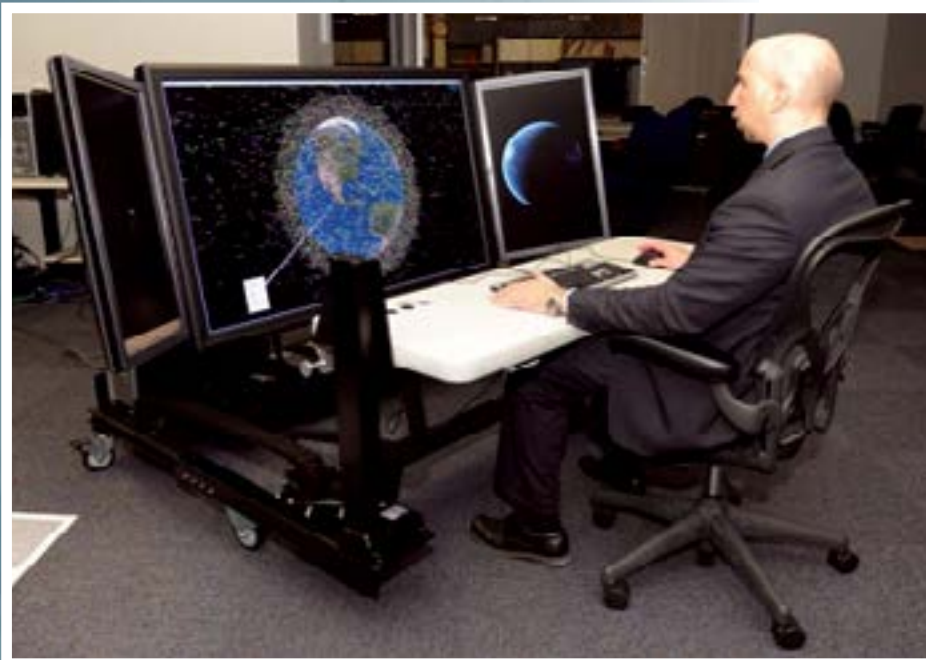
This ergonomically designed large-display workstation is designed for ease of adjustment, portability, and comfort for seated or standing users.
