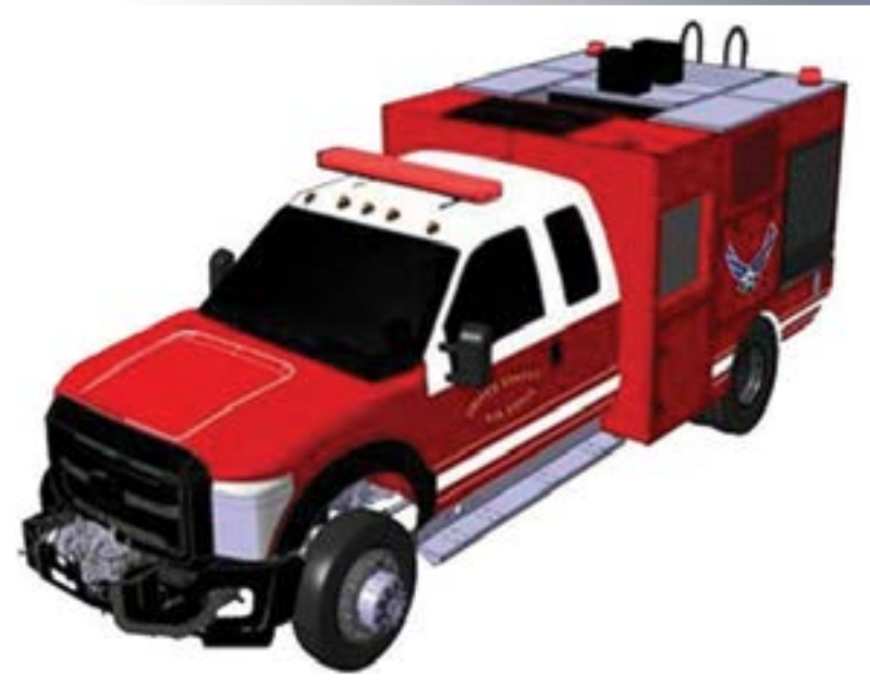
The P-34 Rapid Intervention Vehicle will be the first firefighting vehicle in the AF fleet to use new ultra-high pressure firefighting technology, which is three times more effective than conventional methods.
