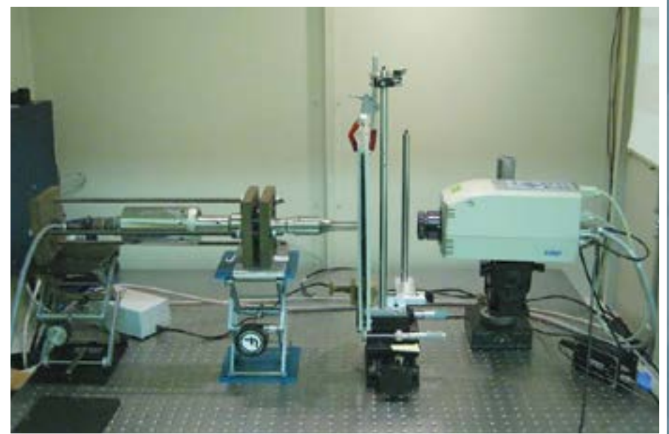
The noncontact thermoplasting property measurement and imaging system setup.
