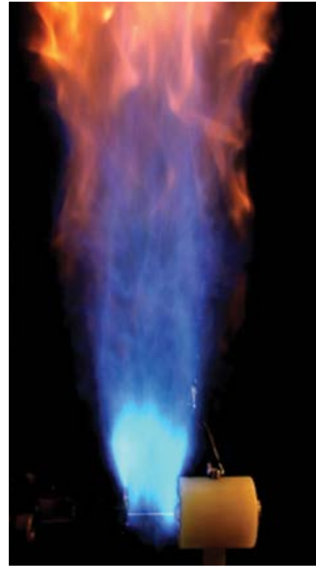
This photograph, exposed over several milliseconds, shows both the laser-induced spark and the subsequent ignition of the flame.
