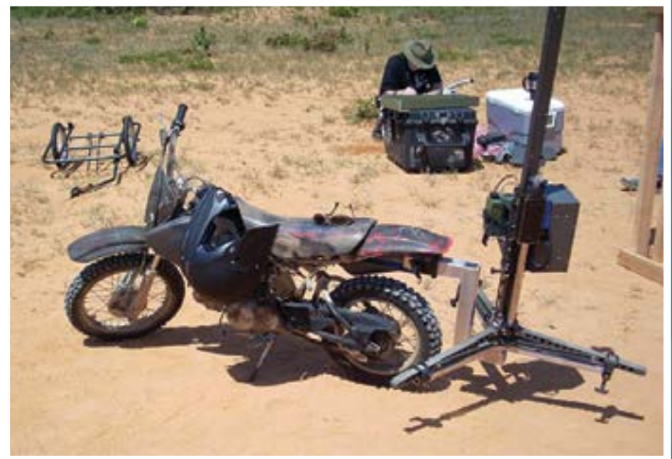
A small bike equipped with a removable hitch for a Mosquito, which provides the capability to measure ground hardness, a crucial element to landing zone preparation.
