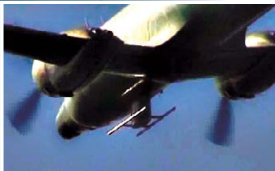
A flight-worthy VHF SAR antennas was tested on a C-131 Aircraft.
