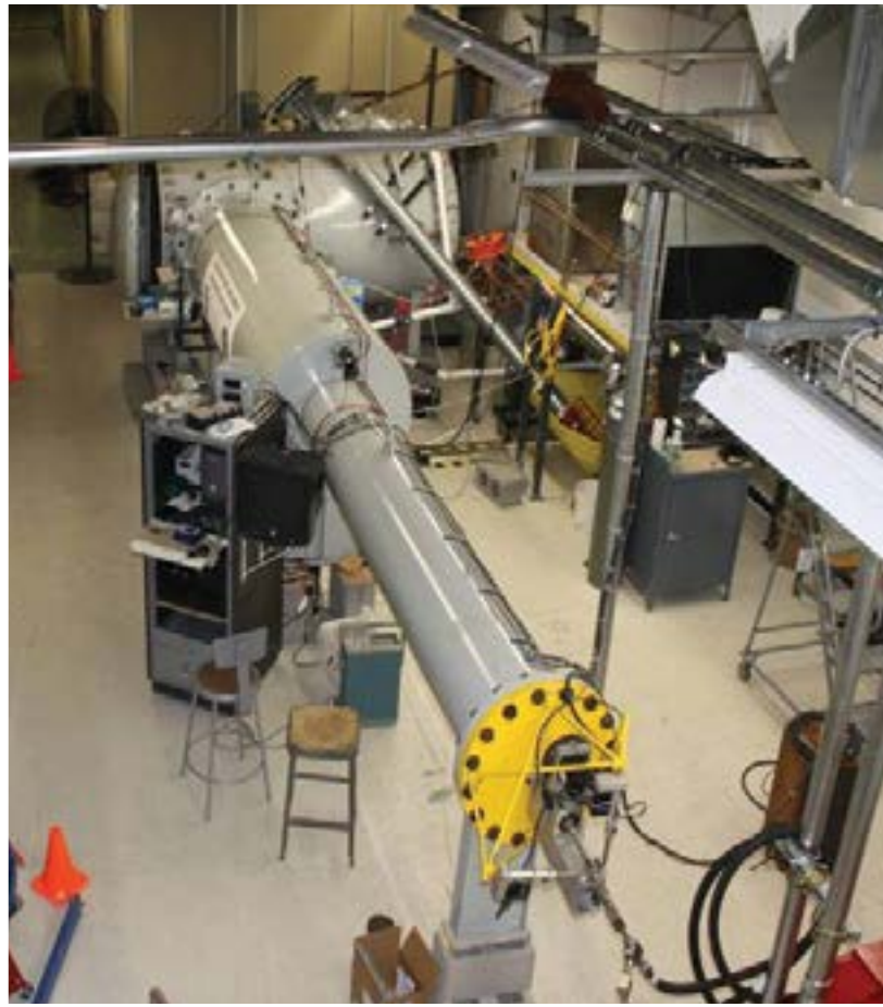
The supersonic rain erosion testing apparatus at AFRL's Coatings and Technology Integration Office simulates the impact of rain on aerospace systems traveling at transonic and supersonic speeds.
