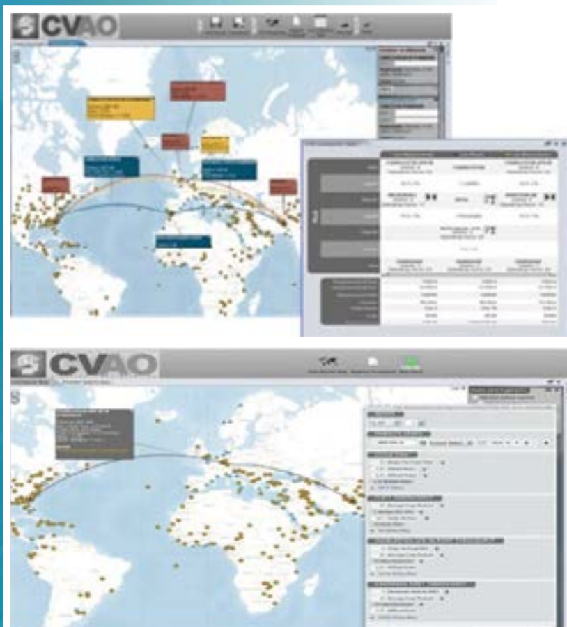
RCAT allows the Fusion Center to easily compare Transportation COAs by initial arrival date, mission count, cost and closure time. (pictured top) Fusion Center Planners can easily view and modify RCAT planning factors such as aircraft cycle time and throughput, resulting in more accurate COAs. (pictured bottom)
