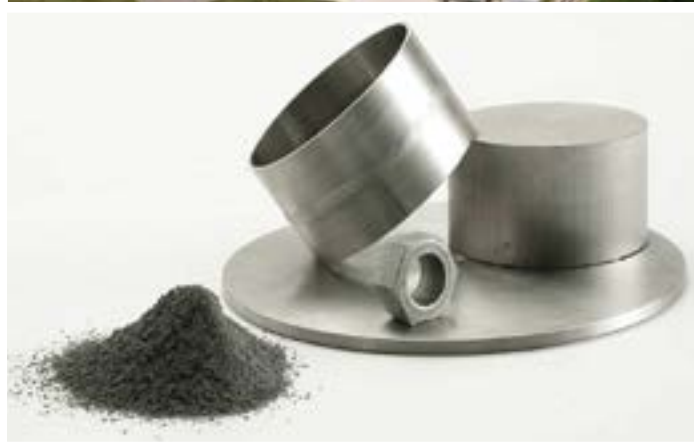
International Titanium Powder's production facility in Ottawa, Illinois. Funds from a Title III program contributed to the construction of equipment. (pictured top) Low-cost titanium powder and titanium parts. (pictured bottom)
