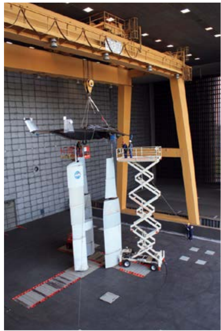
AFRL researchers are testing this 23% scale model of the Speed Agile vehicle at the Arnold Engineering and Development Center's National Full Scale Aerodynamics Complex, the world's largest wind tunnel.
