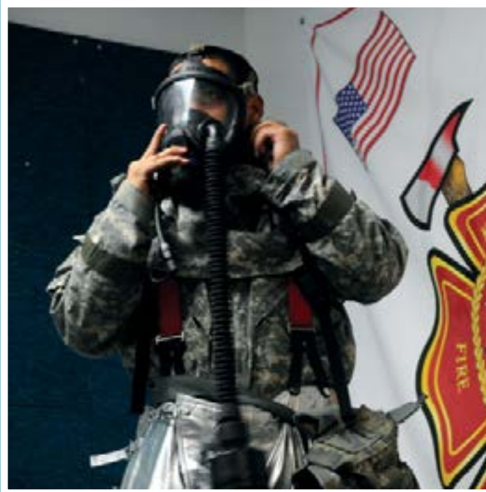
Staff Sgt. Timothy Cruz practices donning and doffing procedures with the new Joint Firefighter's Integrated Response Ensemble. Airmen participated in a final field evaluation of the suit testing the time to put on the JFIRE suits versus the previous version.
