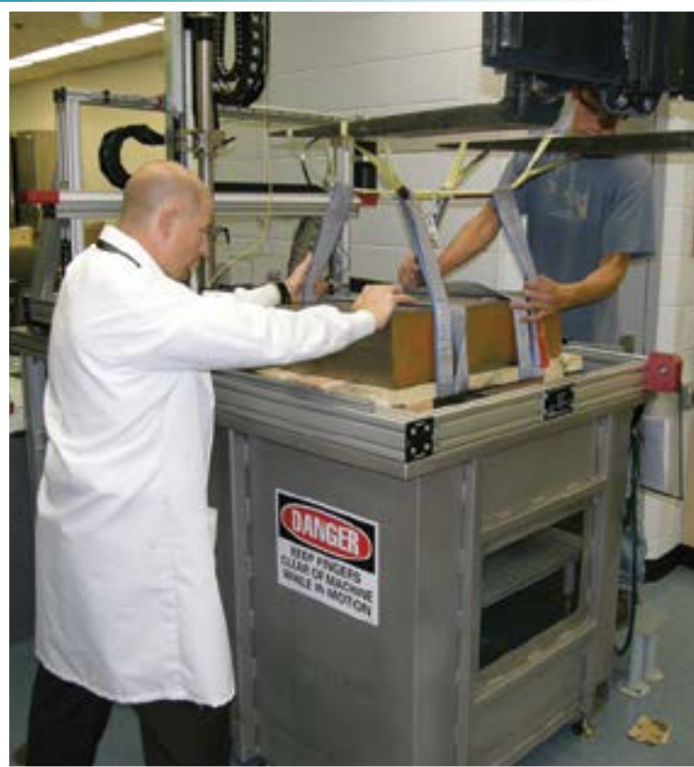
Engineers from the AFRL load a titanium billet for ultrasonic testing, evaluating the substandard material that posed a possible threat to flight and operational safety.
