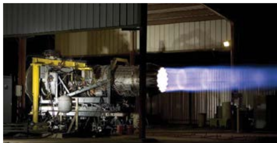
Pratt & Whitney's F135 engine for the F-35 Joint Strike Fighter at test.
