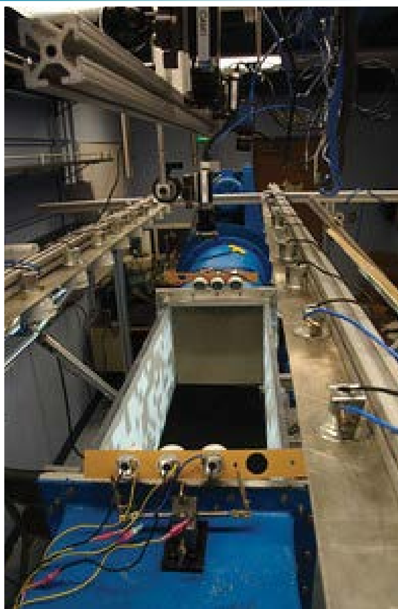
A virtual reality tunnel for fruit flies allows simultaneous tracking of freely flying flies and computer-projected imagery on the walls and floor of the arena.
