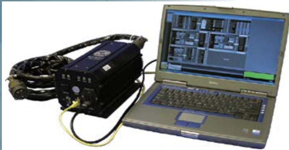
The Legacy Platform Weapon Integration enables direct interface and communication between the Navy Surface Warfare Center and AF BRU-61/A carriage system and SDB stores.
