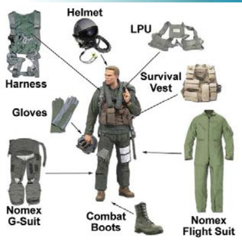
An artist's depiction of the layers of flight equipment worn by a typical Air Force pilot, resulting in complaints of heat-related fatigue from pilots and the idea for a wearable cooling vest.
