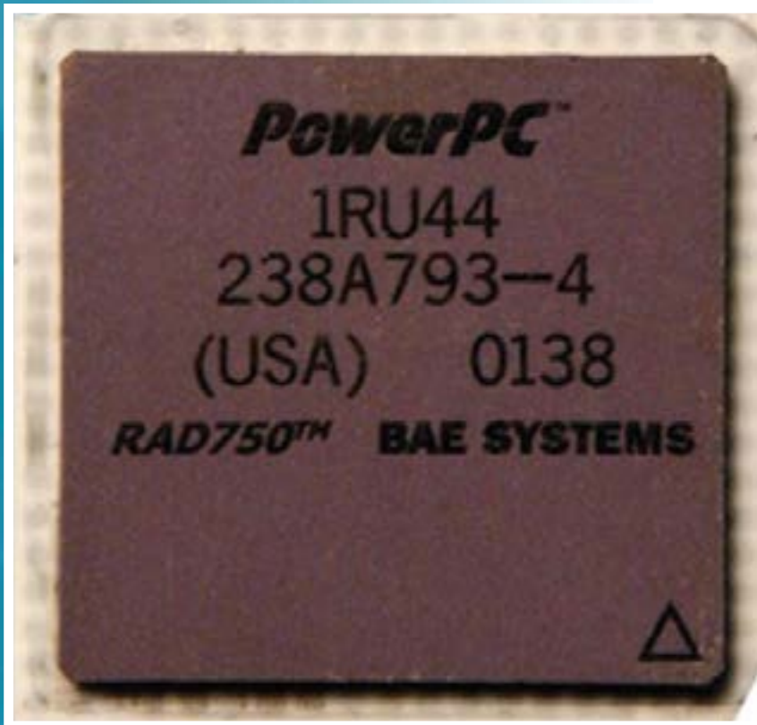
This radiation-hardened microchip enables spaceship operations to survive in harsh environments.
