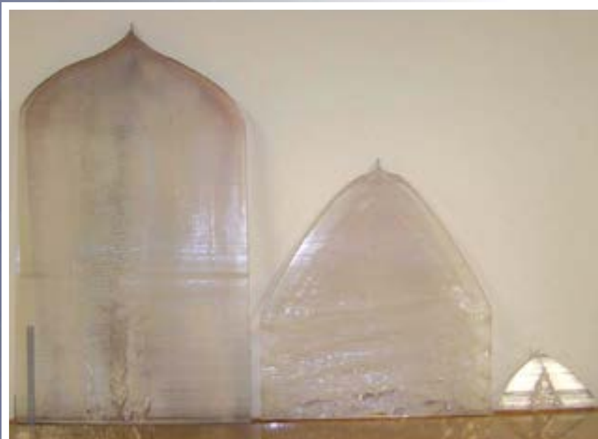
Collaborative work by AFRL and Saint Gobain Ceramics and Plastics Inc. developed new manufacturing processes that increase the size and thickness of sapphire sheets (shown) for electro-optic and infrared windows.
