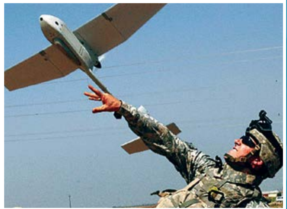
An Air Force warfighter launches a Raven, which will experience increased flight time and endurance thanks to an AFRL partnership that developed lightweight, flexible, high-efficiency solar cells that will adhere to the UAVs wing.
