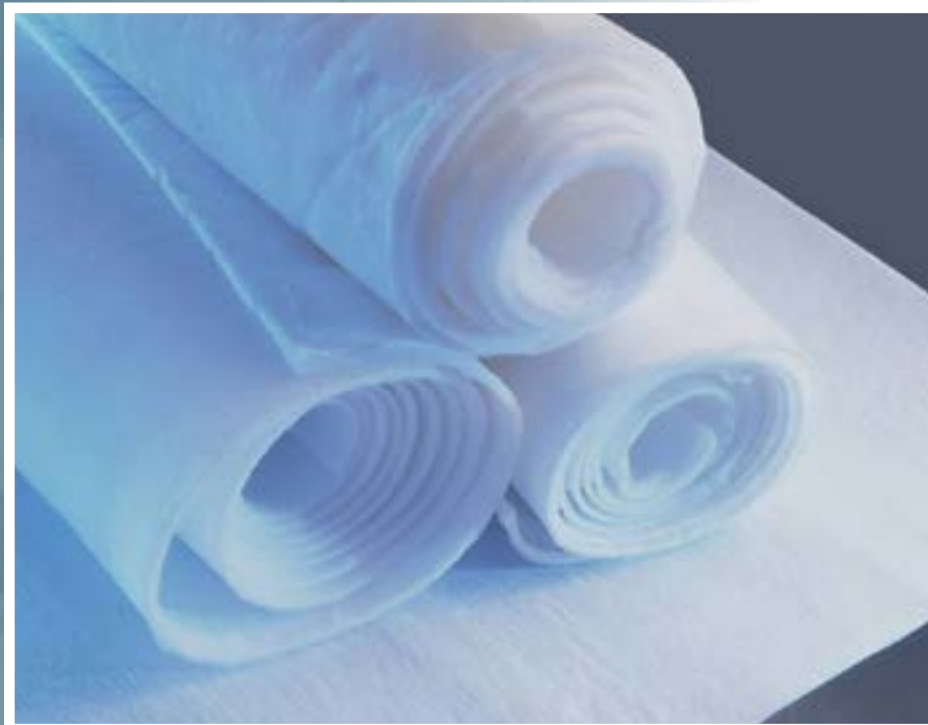
Flexible aerogel, whose nanoscale lattice structure and pores create unique properties in solid material that make it an incredible insulator.
