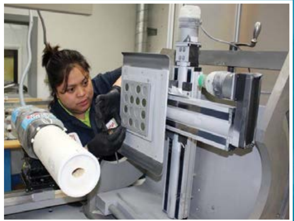
The particle erosion test apparatus, located at AFRL's Coatings and Technology Integration office, aggressively evaluates materials used to protect leading-edge blades in hot, sandy conditions.
