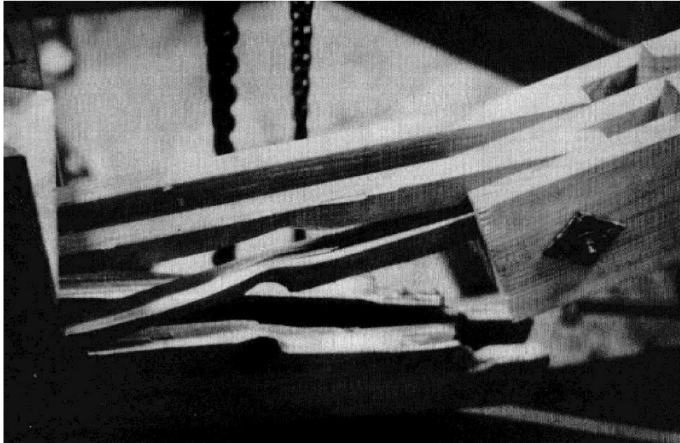
(A) INITIAL SPLICE FAILURE
