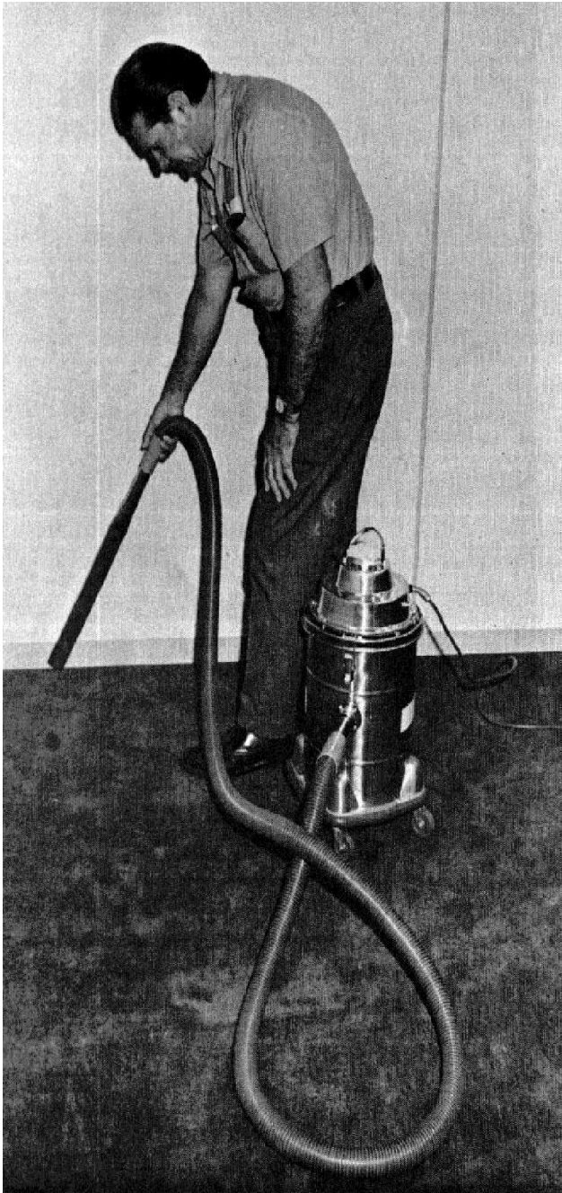
Figure E-7. Wet/dry tank vacuum.
