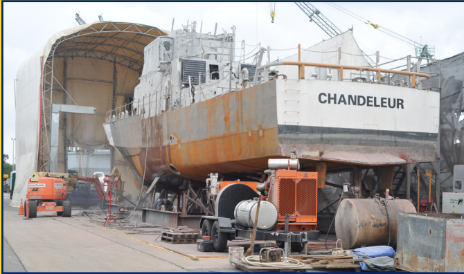
The Coast Guard Cutter Chandeleur, a 110-foot Island-class patrol boat, is drydocked in the Coast Guard Yard at Curtis Bay, Md., to undergo major refurbishing as part of the Mission Effectiveness Project. U.S. Coast Guard photo.
