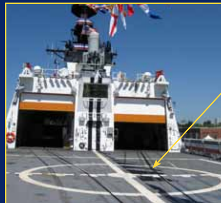
Shown here is the ASIST system track aboard the newest NSC, USCGC Waesche. U.S. Coast Guard photo by Linda M. Johnson
