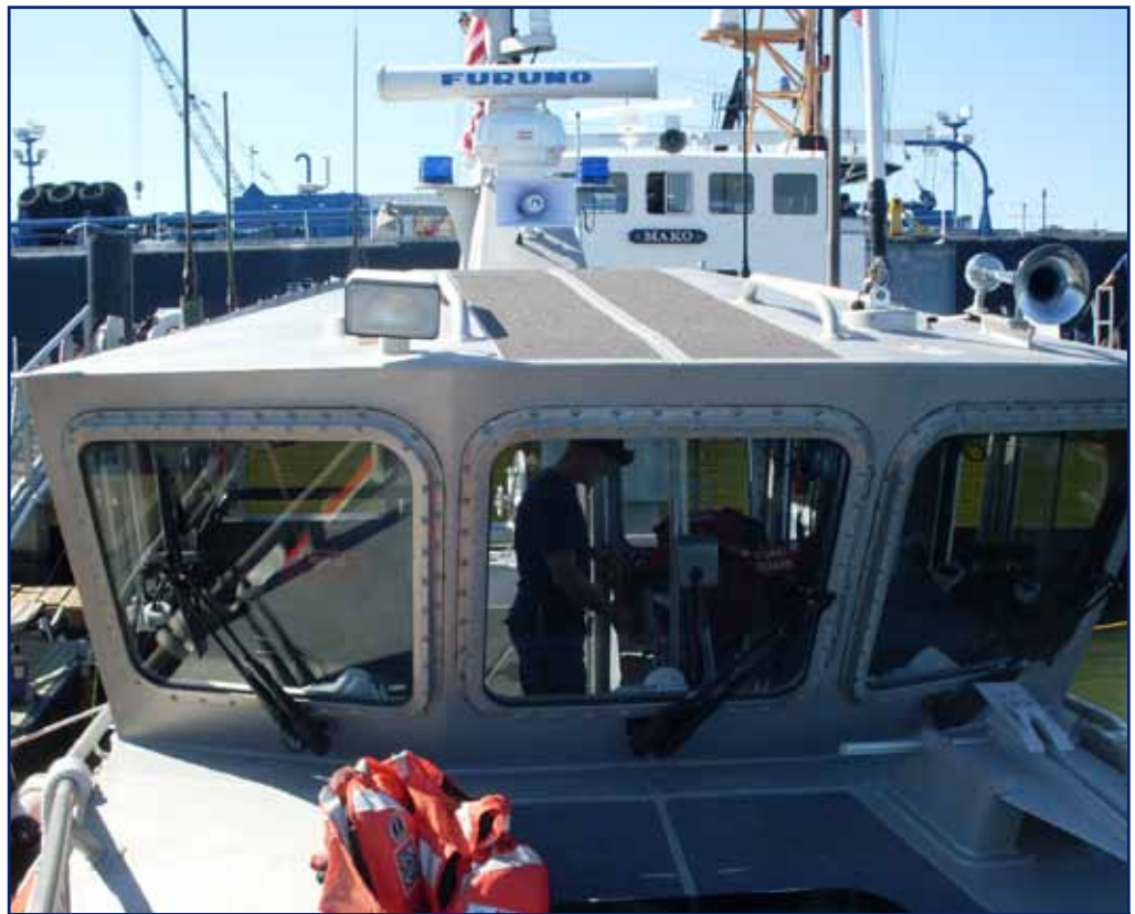
Human factors engineering applied non-skid decals and added grab rails to the cabin roof of the Response Boat-Medium to enhance operator safety when performing routine maintenance. U.S. Coast Guard photo
