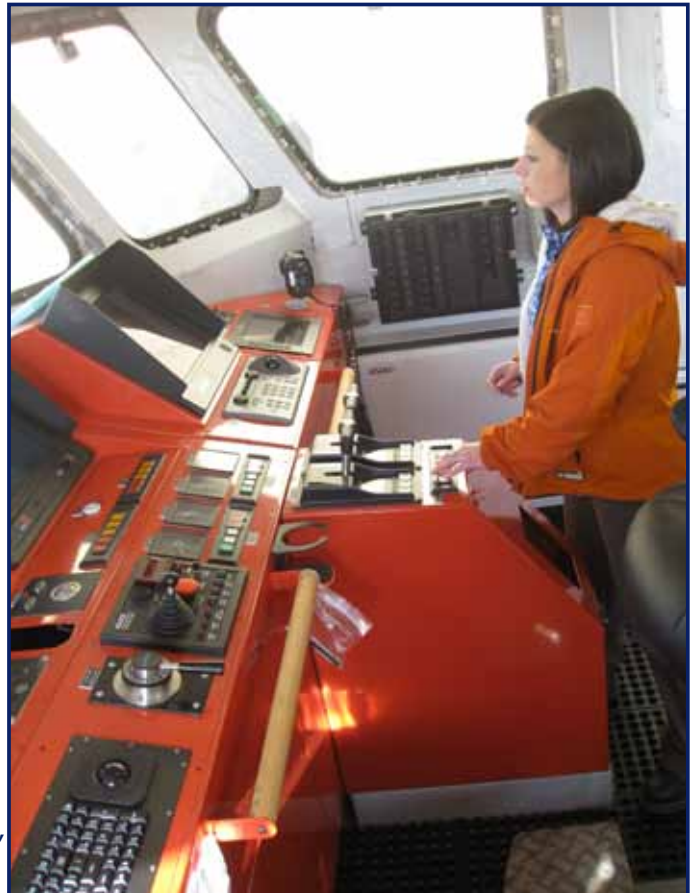
Dawn Gray with the Coast Guard’s human factors engineering team reviews the bridge mock-up for the first Sentinel-class Fast Response Cutter. The mock-up review identified some necessary changes that were incorporated into the bridge design. U.S. Coast Guard photo by Chris Kijora
