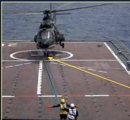
A Republic of Singapore Air Force Super Puma takes off from the flight deck of the Republic of Singapore Ship Resolution, an Endurance-class tank landing ship. The ASIST system is visible in the foreground. U.S. Navy photo
