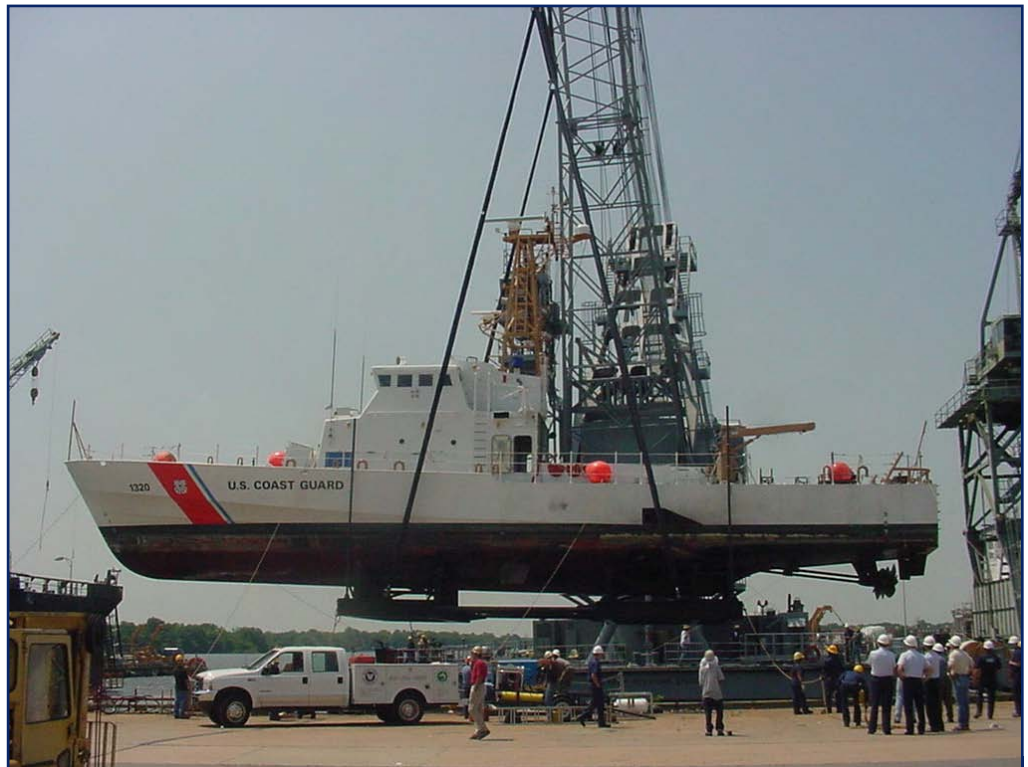
Twenty of the 110-foot Island-class patrol boats, like the one being lifted here, are expected to undergo critical structural and equipment repairs at the Coast Guard Yard as part of the Mission Effectiveness Project. U.S. Coast Guard photo
