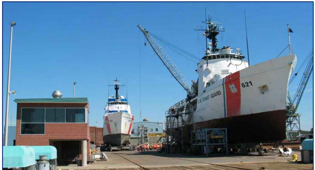
The 210-foot Reliance-class medium endurance cutters Resolute and Valiant are shown undergoing a seven-month major systems refurbishment at the Coast Guard Yard near Baltimore as part of MEP. U.S. Coast Guard photo
