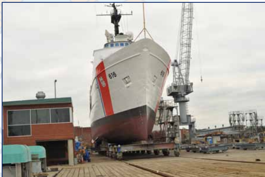
The Coast Guard Cutter Diligence, a 210-foot Medium Endurance Cutter, undergoes major refurbishment at the Coast Guard Yard in Baltimore as part of the Mission Effectiveness Project. U.S. Coast Guard photo.
