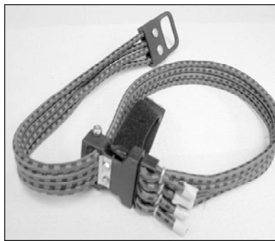
Fig 5. The OHT by Hemodyne. Tension is created by pulling the free end through the metal jaw. This tightens but also narrows the four elastic cords. The silver plate acts to prevent the cords from slipping, but makes it very difficult to release the device.
