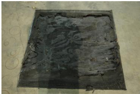
(e) – 5 mm Gasoline Layer Burning Duration = 140s Char Depth = 1–2 mm
