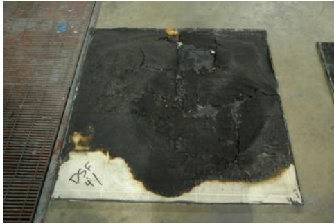
(a) – 1 mm Gasoline Layer Burning Duration = 55s Char Depth = Not measureable
