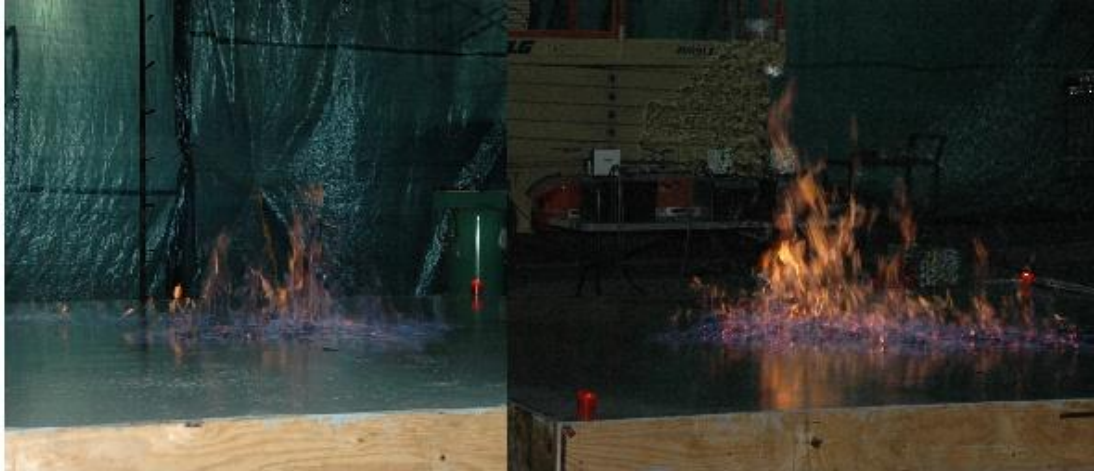
Figure 4.20. Pictures of representative 0.5 L (SFD16-U-CC-DA-0.5-30, Left) and 1.0 L (SFD17-U-CC-DA-1.0-30, Right) denatured alcohol spill fires on coated concrete
