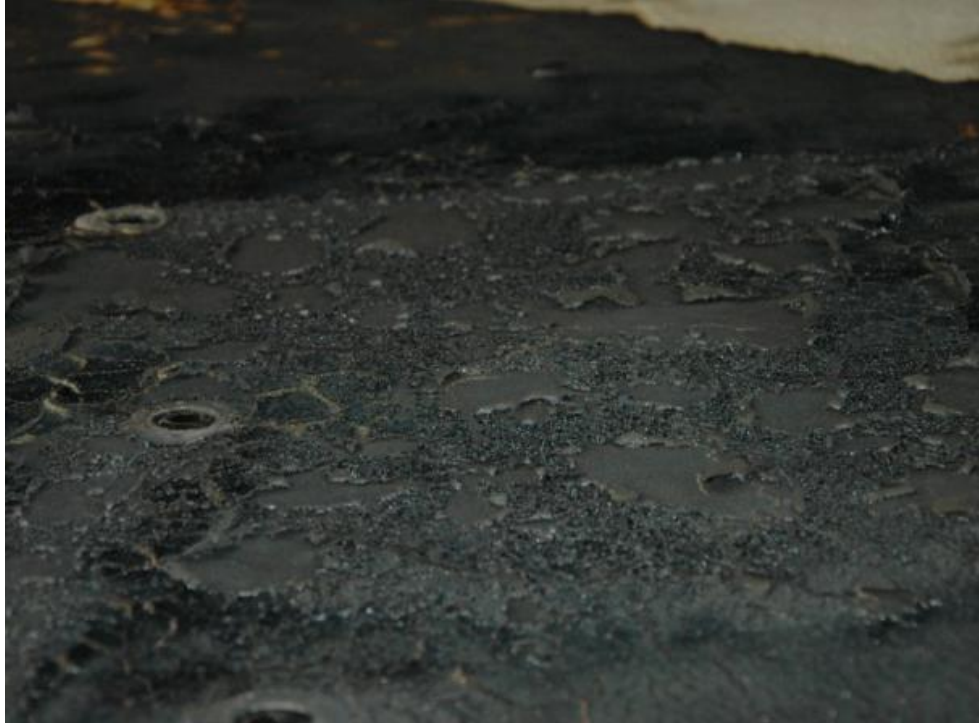
(a) – Degradation of Vinyl due to Gasoline Spill
