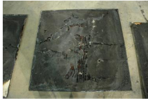
(b) – 2 mm Gasoline Layer Burning Duration = 75s Char Depth = Not measureable
