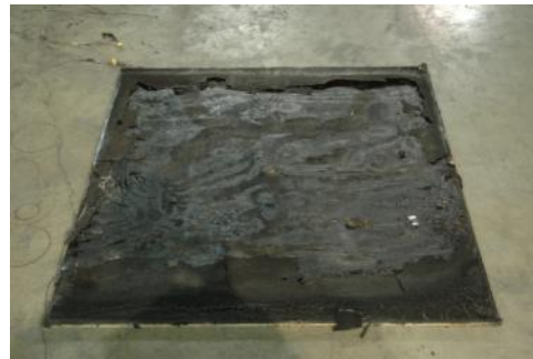
(f) – 20 mm Gasoline Layer Burning Duration = 315s Char Depth = 4–5 mm
