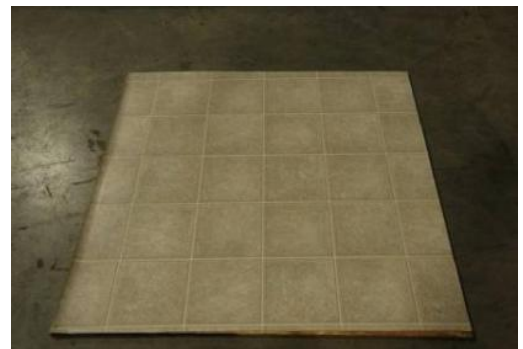
(g) – Vinyl on Plywood
