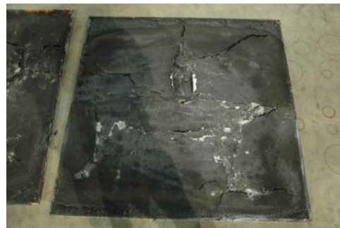
(d) – 4 mm Gasoline Layer Burning Duration = 140s Char Depth = 1–2 mm
