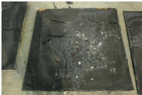
(c) – 3 mm Gasoline Layer Burning Duration = 110s Char Depth = 1–2 mm
