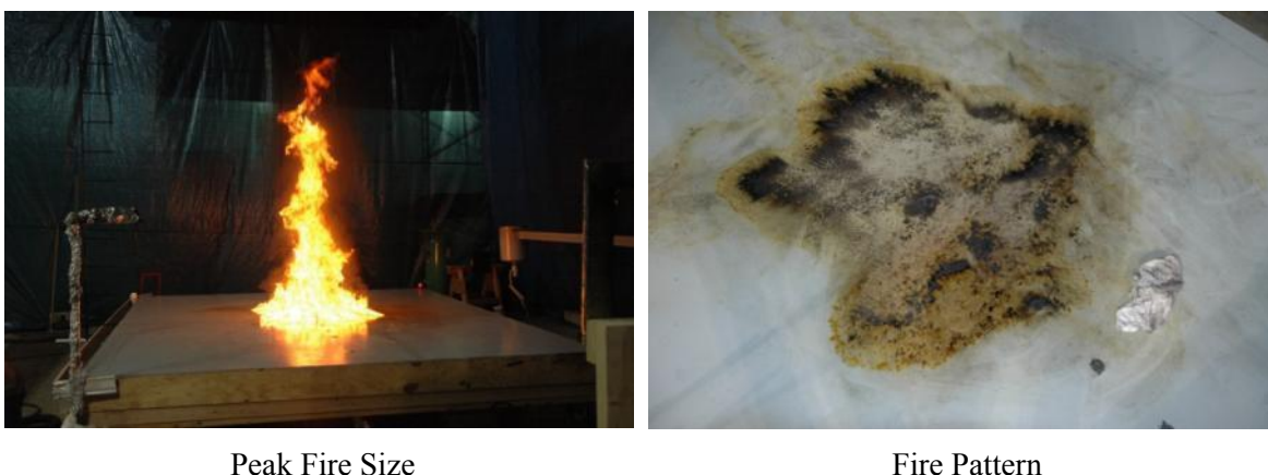
Figure 6.18. Photographs of peak fire size and resulting fire pattern from gasoline on coated concrete (SFD-U-CC-G-0.5-30)
