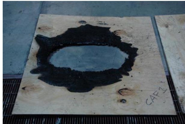
Wood Crib (Note: Carpet/padding layers have been removed.)
