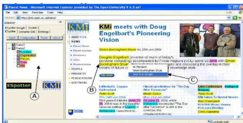
Fig. 1. ESpotter highlighting a page on the KMi Web site [4], showing (A) the ESpotter toolbar (B) entities highlighted according to their types on the Web page (C) services provided for entities (such as search for them in Google).
