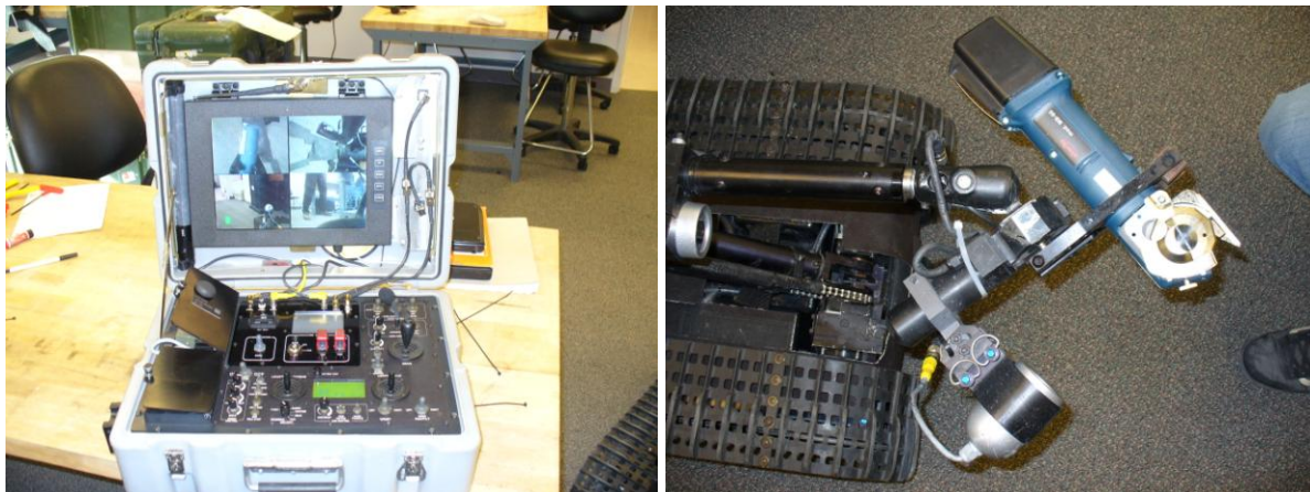
Figure 5: Trial Cordless Cutter Mounted On TALON Checking For Camera Angles And Control
