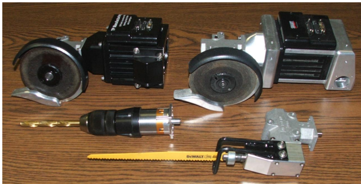
Figure ES-4: Whether Configured For Andros (Left), Landshark (Right) Or Any Other Platform The Dervish Can Be Fitted With All Tool Options.
