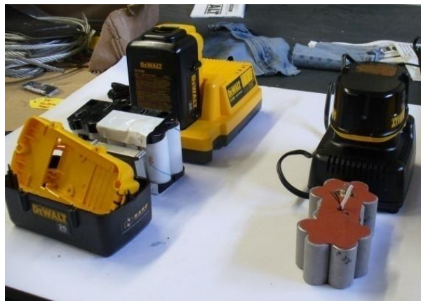
Figure 45: COTS Batteries Come With Smart ‘Fast’ Chargers And Can Be Used In Original Housings Or Stripped Out And Repackaged.
