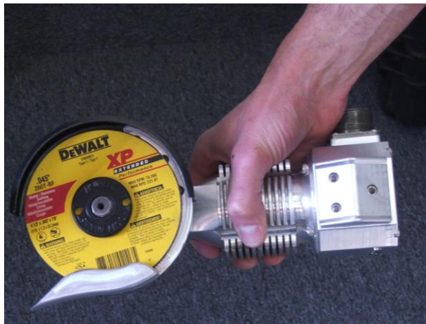
Figure 48: While Not Optimized For Hand Use The Low In-Hand Weight Means Either Dervish Can Be Easier To Utilize Than Conventional Tools For Short Occasional Uses.
