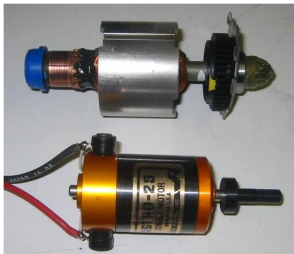
Figure 15: 85% Efficiency A-90 Motor (Bottom) In The Same Form Factor As The DC410 Motor (Top).
