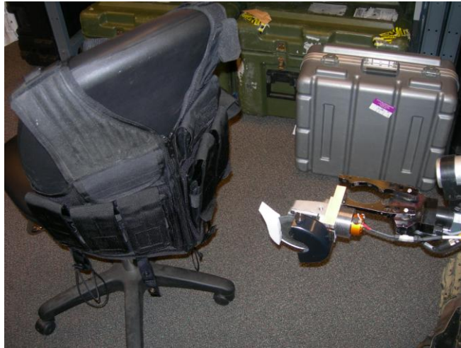
Figure 7: Cutter Positioned On The Outside Of A Pincher Gripper Of The TALON
