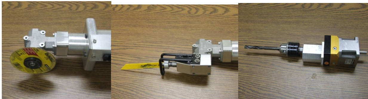
Figure 59: The Core Dervish Power Unit Can Be Fitted With Small Cutting Disc, Breaching Disc, Reciprocating Saw And Drill.
