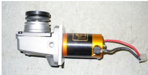
Figure 27: A90 Motor Adapted To The DC410 Right Angle Drive With Heat Shield Removed
