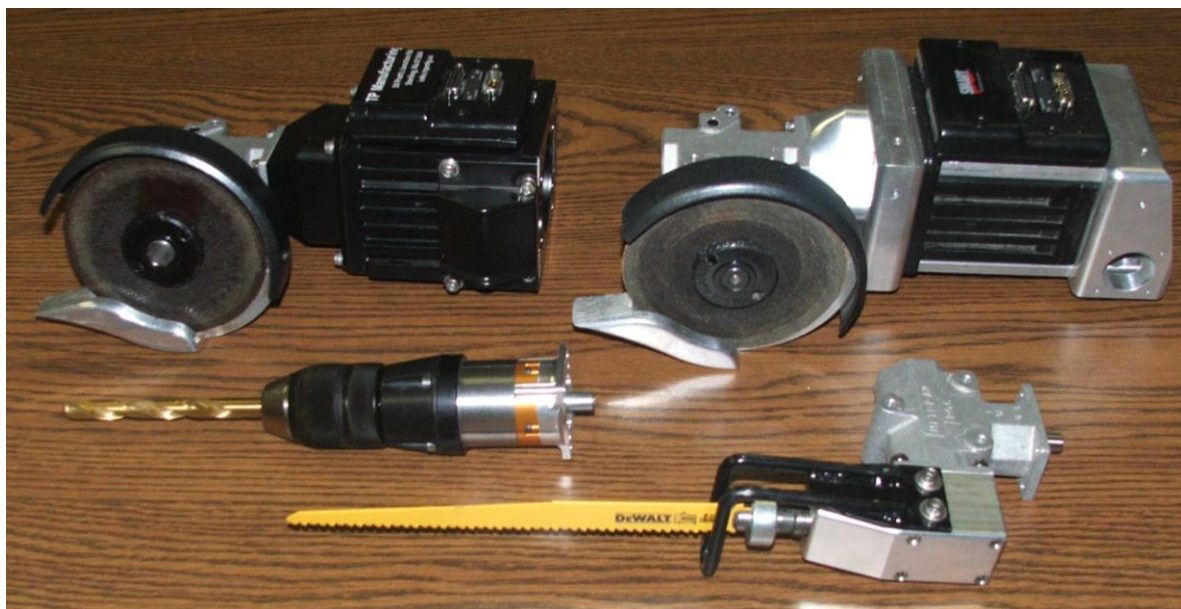
Figure A-4: Whether Configured For Andros (Left), Landshark (Right) Or Any Other Platform The Dervish Can Be Fitted With All Tool Options.
