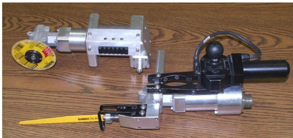
Figure 56: The Dervish Power Unit Fitted With A Landshark (top) and TALON (bottom) Manipulator Interface Kit (And Reciprocating Saw Discussed In Section 3.1.1.5).
