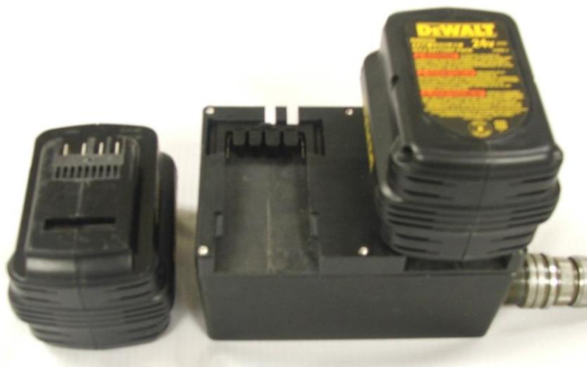
Figure 46: COTS Batteries Mount To The Dervish Electronics Box Through Their Standard 'Tool' Interface.
