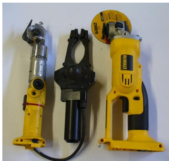
Figure 14: Cordless Rug Cutter, TALON Gripper, And Dewalt DC 410 Cordless Grinder Without Batteries
