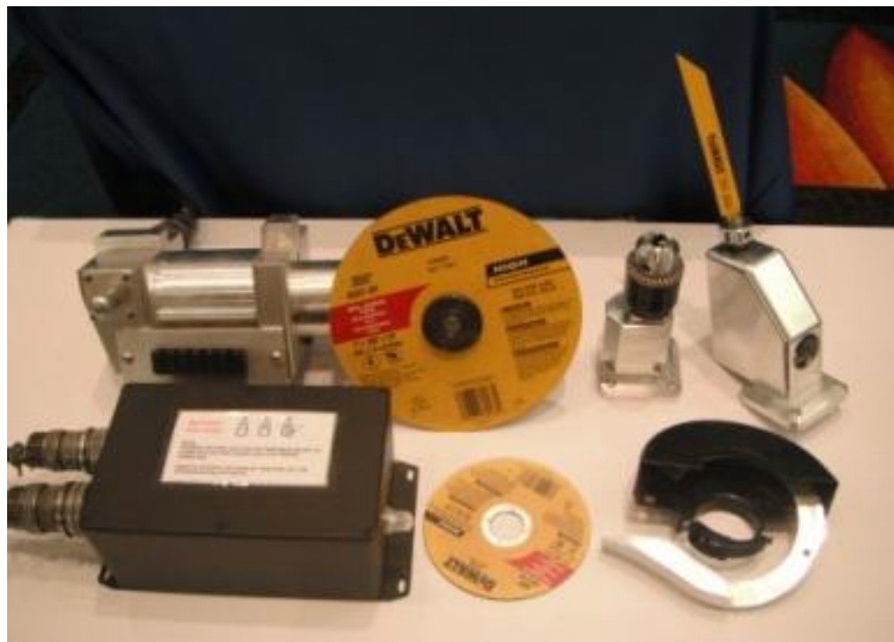
Figure 3: The Dervish Is A Family Of Tool Heads That Mount To A Drive Unit With Dedicated Power And Controls.
