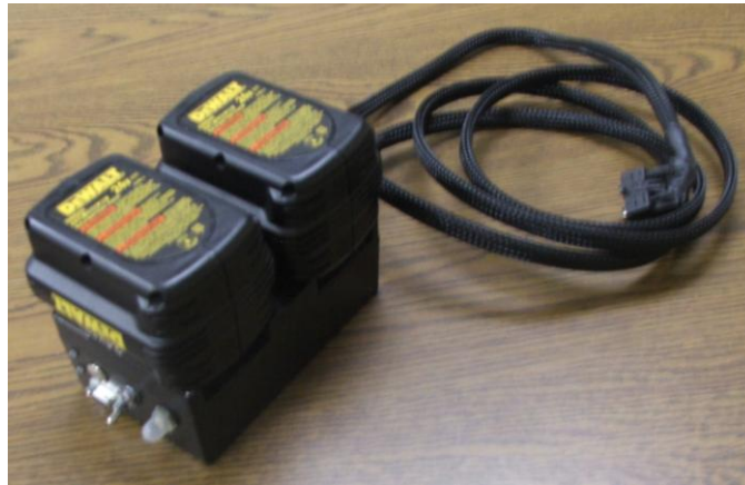
Figure A-7: The Battery/Electronics Box Has Shrunk Considerable From Phase II And Incorporates The Simplistic Operator Controls.
