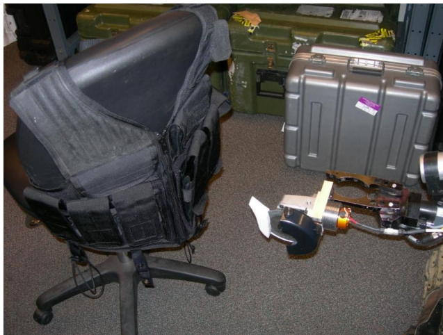
Figure 35: The TPI Cutter On The Foster-Miller TALON System Cutting A Tactical Vest Hung From A Chair.
