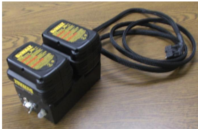
Figure ES-5: The Battery/Electronics Box Has Shrunk Considerable From Phase II And Incorporates The Simplistic Operator Controls.
