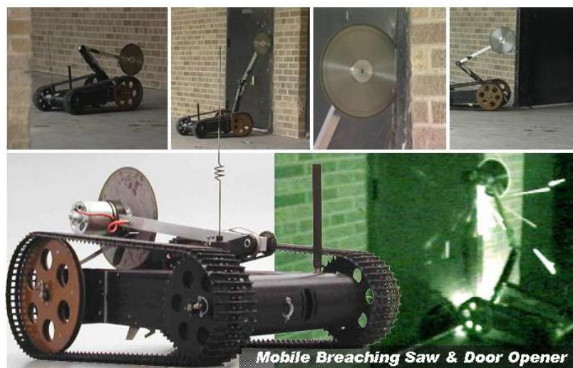
Figure 38: Door Breachers Have Been Implemented On Robots Before But Only As Semi-Permanent Integrated Tools.
