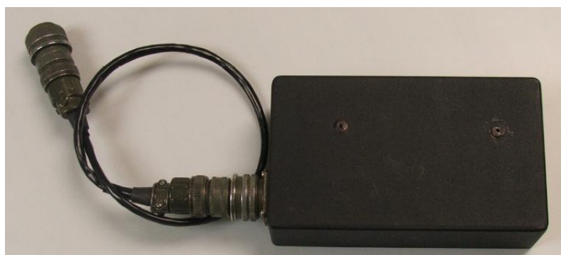
Figure 43: A 48-V Battery Pack Supports High Power Draws And Longer Missions.
