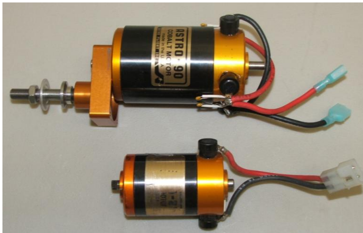
Figure 51: Dervish Was Upgraded To A New High Power, High Torque Motor (Top Motor) With Integral Gear Reducer.
