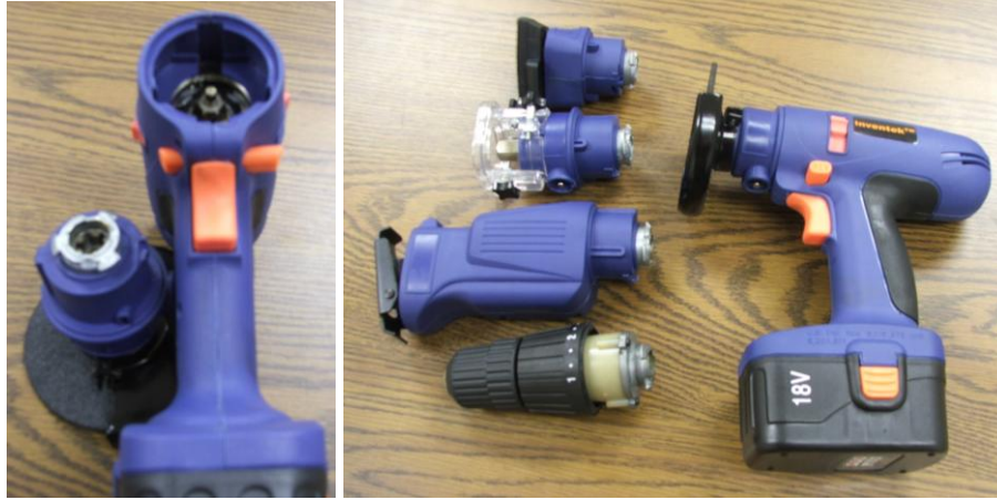
Figure 57: COTS Systems Are Available That Feature Interchangeable Tool Heads For Drills, Reciprocating Saws, Grinding Wheels, 'Roto-Zip' Heads And Vibrating Sanders.
