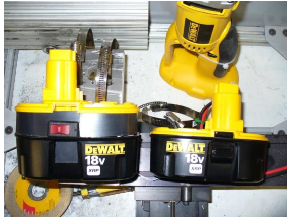
Figure 25: Circuit Board Only Added About ¼-In In Thickness To The DC410 (Left) Compared To Unmodified System (Right)
