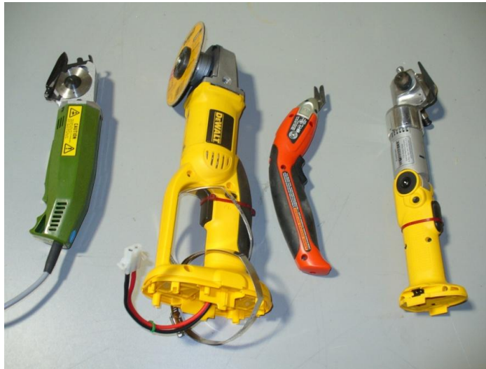
Figure 10: Tested Cutters - AC Powered Textile Cutter, Battery Operated Grinder, Battery Operated Snips, Battery Operated Textile Cutter. Not Shown Are The Bosch/Emery Units.
