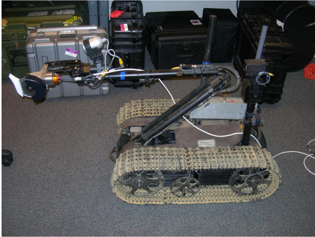
Figure 29: Dervish With Separate Power Head And Battery/Controls Package Mounted On TALON
