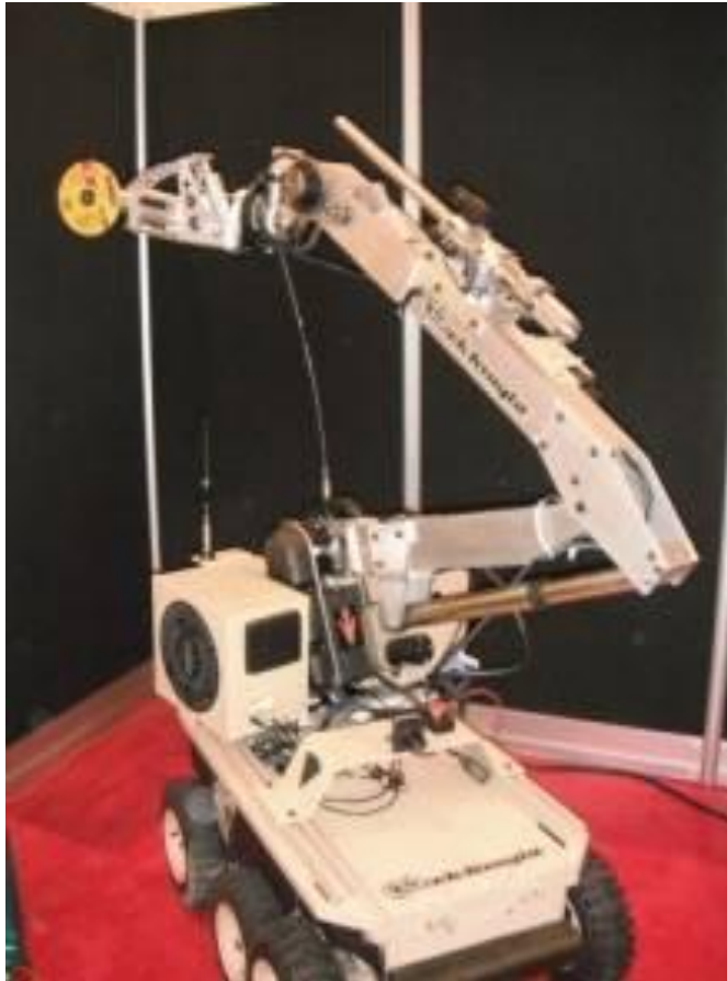
Figure 54: The Dervish Power Module Was Fitted With Adaptors To Match The Landshark Manipulator.
