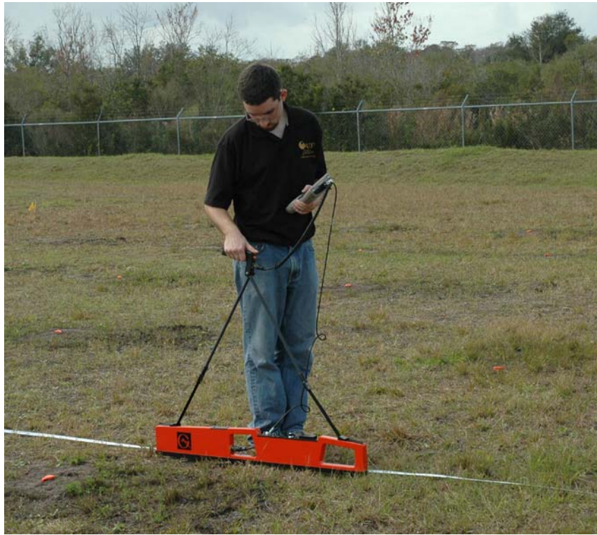
Figure 7-1. Data collection using the Geonics Limited EM-38RT conductivity meter in the vertical dipole along a grid line at the research site.
