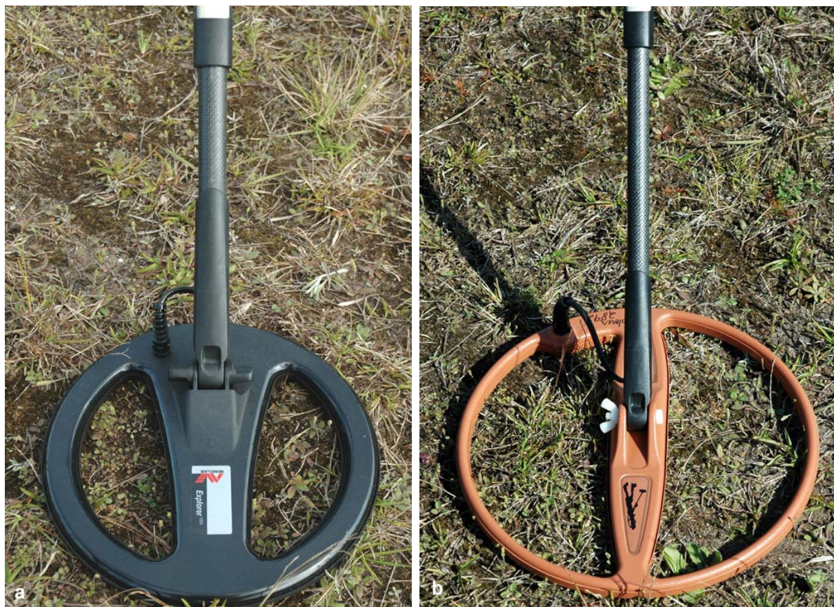
Figure 6-1. Minelab Explorer II™ with (a) medium 10.5 inch (26.7cm) coil, and (b) 15 inch (38.1cm) Coiltek search coil
