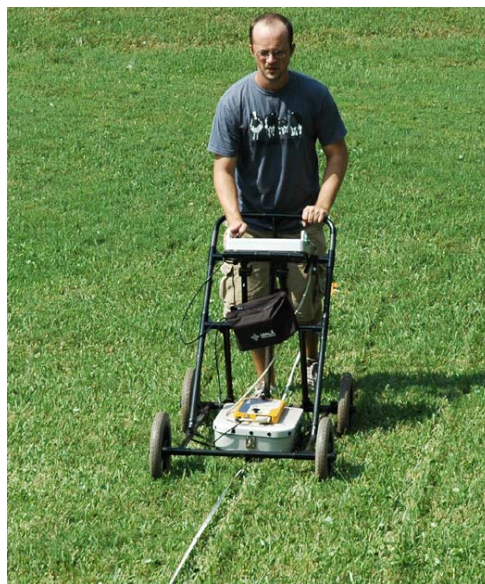
Figure 8-1. MALA RAMAC X3M with GPR unit with 500-MHz antenna integrated into a cart
