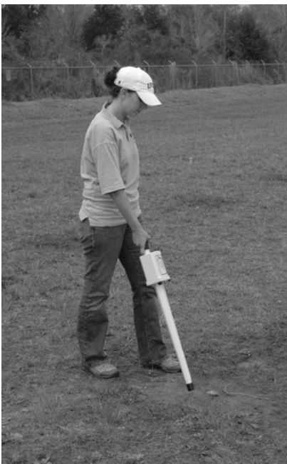
Figure 4-1. Schonstedt GA-72Cd magnetic locator
