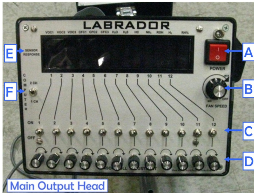
Figure 1. Main Output Head. (A) Power switch. (B) Fan Speed Knob. (C) Individual Sensor Selection Switch. (D) Sensor Null Adjustment Knobs. (E) Sensor Response Display. (F) Computer Interface Summing Amplifier Selector Switch.
