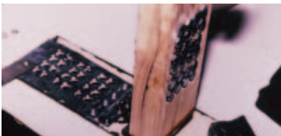
Figure 16a: A homemade punch used by a large-volume meth lab for removing over-the-counter tablets containing ephedrine or pseudoephedrine from blister packs.
