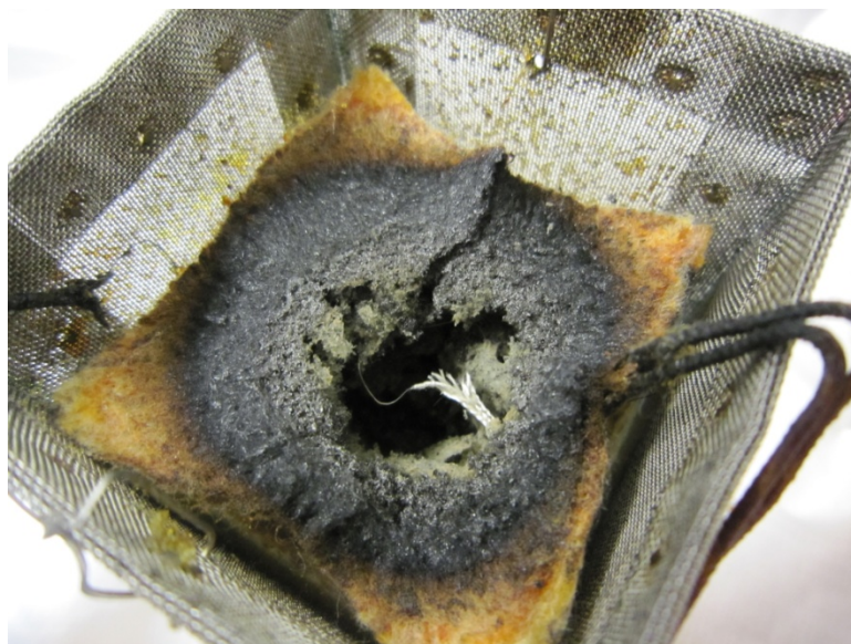
Figure 10. Void space occurs and enhances flaming
