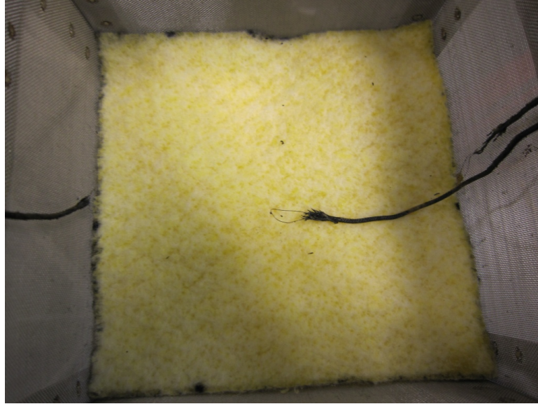
Figure 5: Thermocouple Placement In the Center and On the Surface of the Sample
