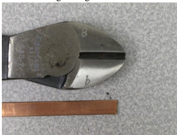
Figure 17: Tool mark on copper sheet
