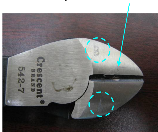
Figure 60: Picture of a tool with engraved label “B” and “b”, and middle mark of the blade.
