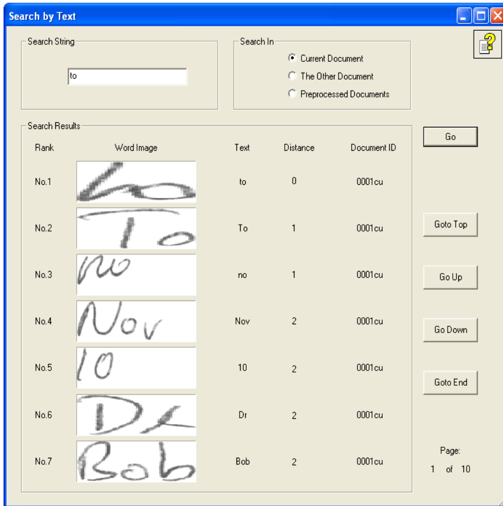
Figure 5: Word Search. The user can type in a search string for which the system will retrieve potential matches in the handwritten document.
