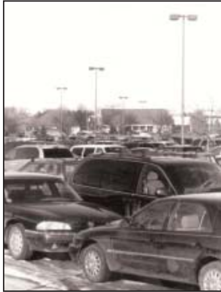
Tall lights provide uniform coverage of a lot and are difficult to vandalize.
