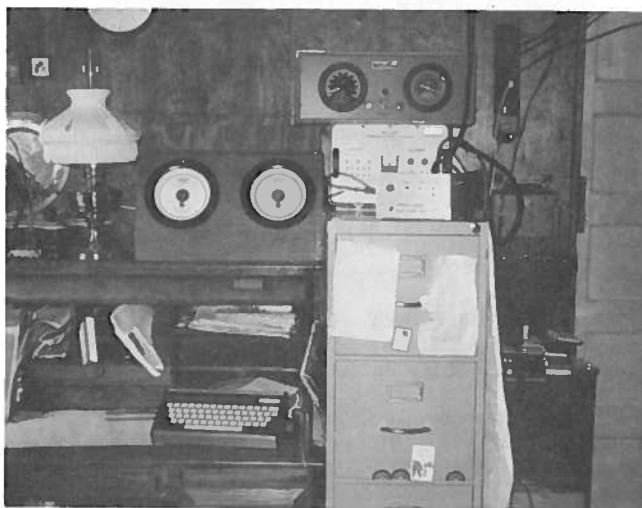
Observers home with wind, pressure, and meteorburst equipment.
