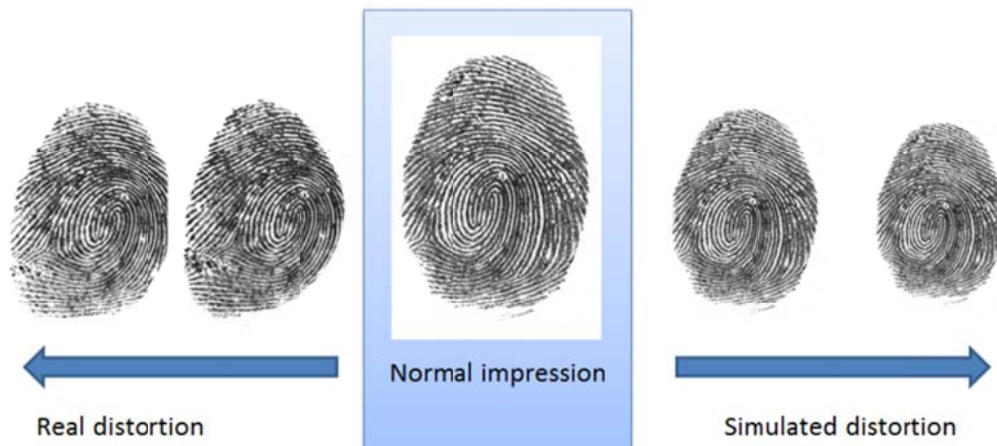
Figure 12: Comparison of empirical and simulated distortion. The 3 images on the left are actual prints that were obtained using our livescan system. The 2 images on the right were generated by applying the skin-distortion model to the normal impression in the middle.
