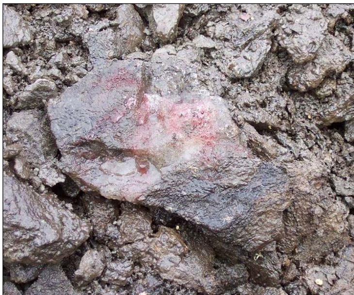
Figure 59. When alpha, alpha-dipyridyl is applied to a soil containing reduced iron, a positive reaction is indicated by a pink or red coloration to the treated area.
