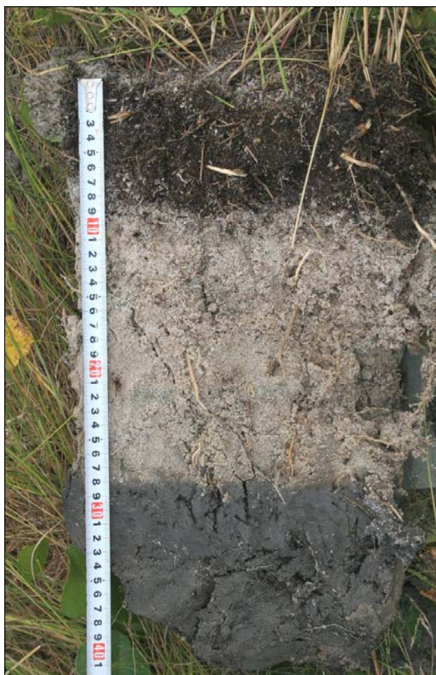
Figure 16. This soil meets indicator S1 (Sandy Mucky Mineral). It also meets indicators S5 (Sandy Redox) and F2 (Loamy Gleyed Matrix). Photo by John Gagnon and John Kelley, NRCS.
