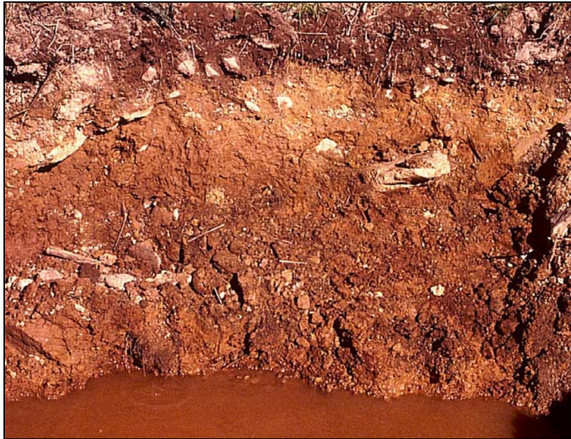
Figure 67. Observing redoximorphic features in soils developed from red parent materials can be problematic.
