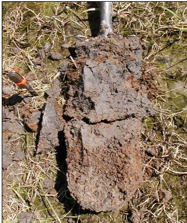
Figure 60. Redox concentrations in the tilled surface layer of a recently cultivated soil.
