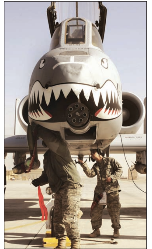
SENIOR AIRMAN WILLARD E. GRANDE II Crew chiefs install pins on an A-10C Thunderbolt II at Kandahar Airfield, Afghanistan. The A-10, one of the aircraft already tested for biofuel blends, has also been the focus of research for battle damage repair.
