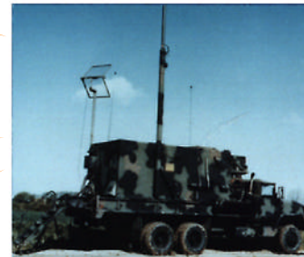
Engagement Control Station
