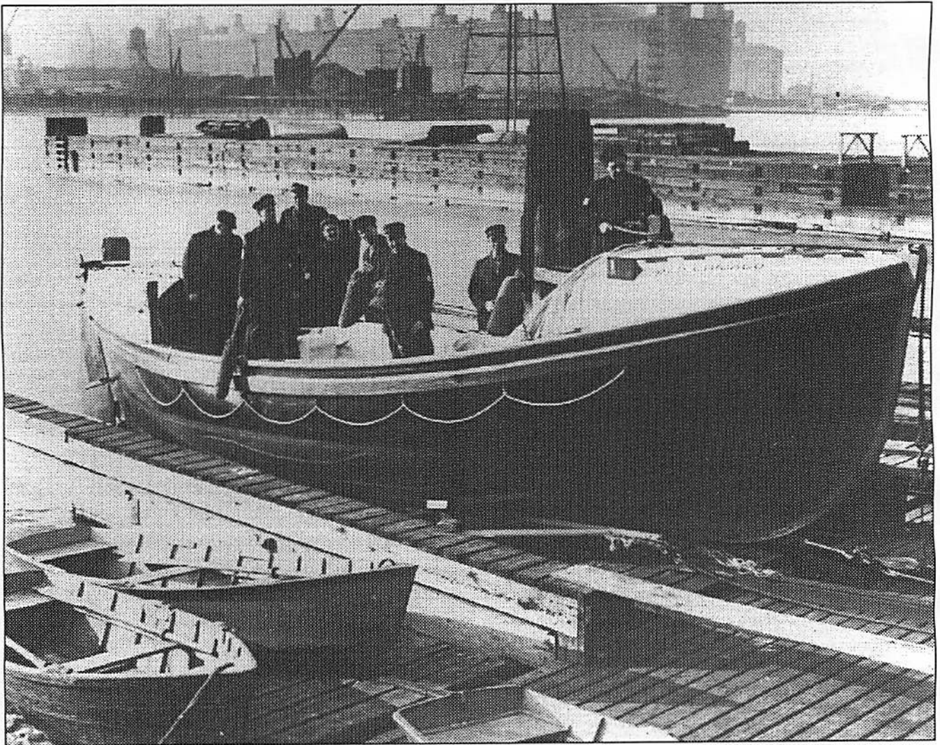
The 36-foot motor life-boat, capable of sail or gasoline power and used by stations all over the country.
