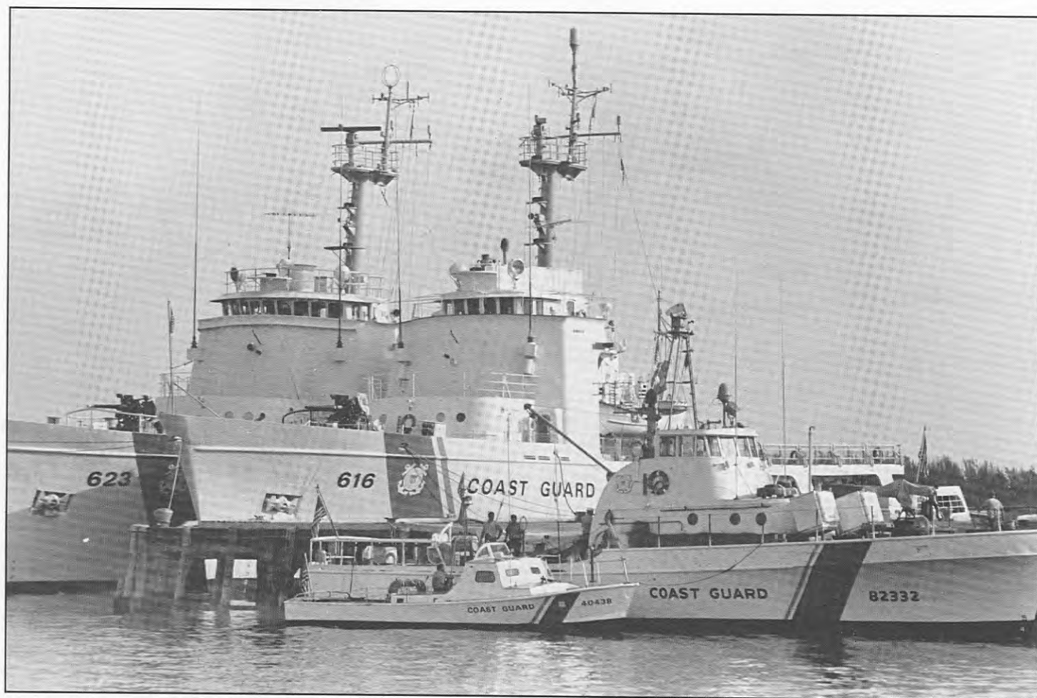
Coast Guard patrol forces in Key West, Fla., 1971, consisted of two 210-foot medium endurance cutters, an 82-foot patrol boat and 40-foot utility boat.
