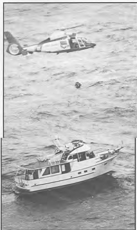
The Service's newest rotary wing aircraft, the HH-65A "Dolphin", prepares to make a basket hoist. One of the greatest improvements in shore-based search and rescue came with the development of the helicopter as a rescue tool.
